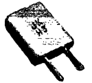
H-3 (HC-18/U Except .039". Pin Dia.) Pin Spacing .192". H-3W (HC-18/U) With Wire Leads
