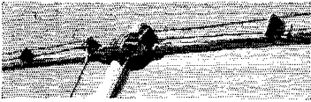
Linear Loading--The new linear loading concept reduces element length and maintains higher efficiency than coil loading.
