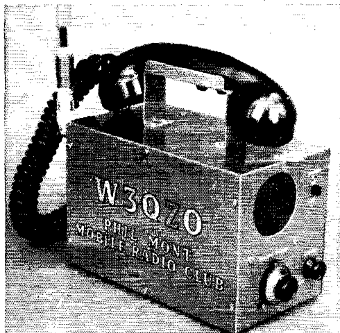
This is the receiver end of the W3QZO walkie-talkie. The speaker behind the circular cutout can be turned on or off with the slide switch beside it. The vernier dial is for receiver tuning, and the other knob is on the combined volume control and power switch. The small aluminum tabs on top of the box at each end are for a carrying strap.
