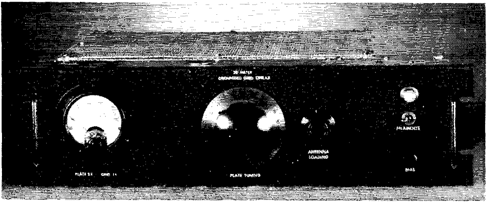
All amplifier units have the same panel design. This unit is the one used for 20 meters. Tuning and loading controls are at the center. The small knob in the lower right-hand corner is for adjusting bias.
