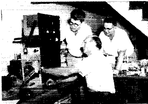
In a typical ARTS session in the basement shack of WØIFC, he demonstrates his "V.h.f. Corner" to WØQHL and KØHZW. Andy is adjusting a 220-Mc. transmitter. In the rack alongside is a 50- and 144-Mc. rig with a pair of 4-65As in the final.
