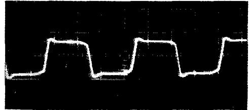
D—30-watt load with the filter in use.
