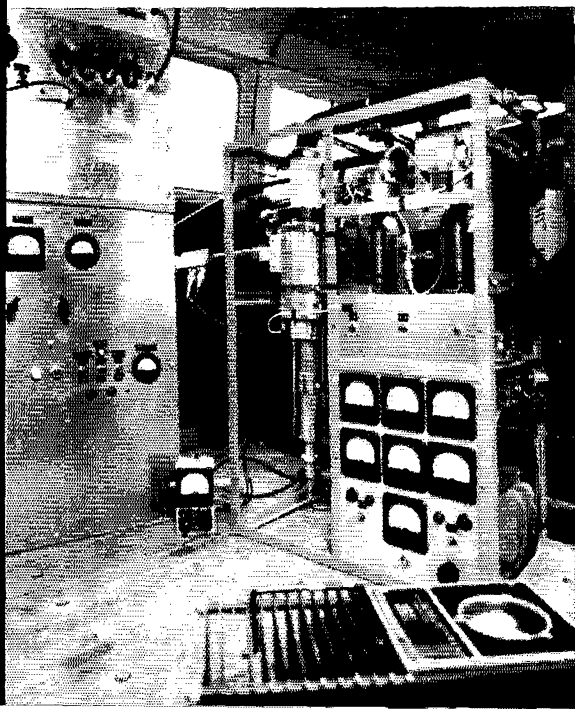
Transmitter used for first 1296-Mc. moonbounce signals received from Europe, via HB9RC, HB9RF and their hard-working group.
