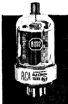
RCA-8032 Beam Power Tube—70 watts CW output (ICAS) at 60 Mc; 35 watts CW output at 175 Mc.
