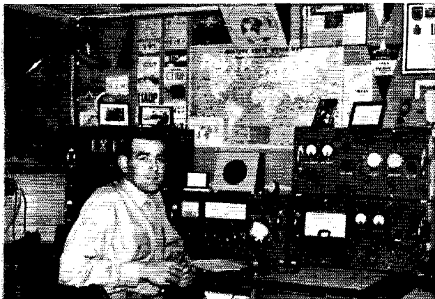
1X1TJ is a delicious 14-Mc. single-side-band morsel also sometimes available on 10 and 15 meters. Jules sports 150 watts, a double-con superhet and a triband quad. (Photo via W3ICQ)
