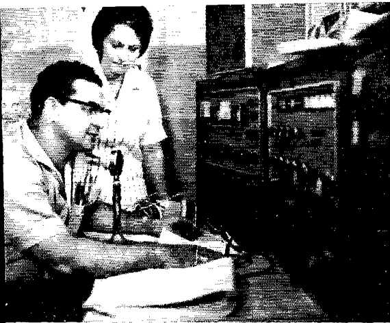
YV6AV/2 and XYL YV2DW punch quite a hole in the 10-, 15- and 20-meter phone ranges with their HK-500, Thunderbolt, HQ-170, cubical quad and TA-36 beam. Johnny and Pat also keep a multiband dipole handy for occasional DXcursions to 40 and 80 meters.
