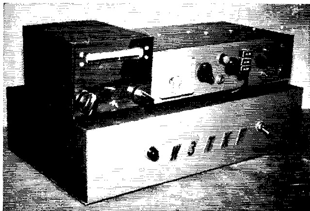
The complete 50-Mc. transmitter at W3TXF. The large base unit contains power supplies and audio equipment. The v.f.o. described here is at the upper left. The transmitter proper is a 10-watt r.f. unit for 50 Mc. taken from the Handbook of some years back.
