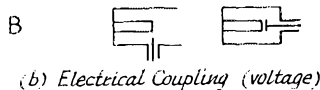
Fig. 3—Approximate voltage and current distribution in one-quarter wavelength (A), one-half wavelength (B), and three-quarter wavelength (C) resonant coaxial lines. The field strength, E , is also shown. At B, an illustration of magnetic and electrical coupling to coaxial cavity circuits.
