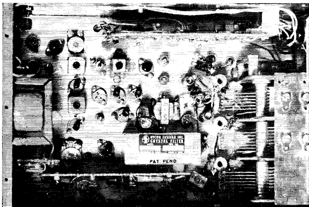
Interior of the 50-Mc. receiver. The 3-gang tuning capacitor, actually at the front of the receiver, is in the right edge of the picture. The circuit board at the lower left carries the bandpass filter circuits. The 10.7-Mc. i.f. and filter circuits are near the center, with the 455-kc. i.f. components in the left center. The circuit board at the upper right has the first audio and squelch components.
