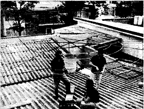
The "circular cylindrical" antenna shown above (l.) was constructed by Raul Mejia M., HK4TA. He reports that the antenna performs well, is resistant to high winds and bad weather. The circular elements are made from 1/2-inch aluminum tubing and are formed on the ground. The lengths are determined by using conventional formulas for quad element lengths. The photograph on the right shows HK4TA, HK4PJ, and HK4BAJ adjusting the antenna with a grid-dip meter and a communications receiver.
