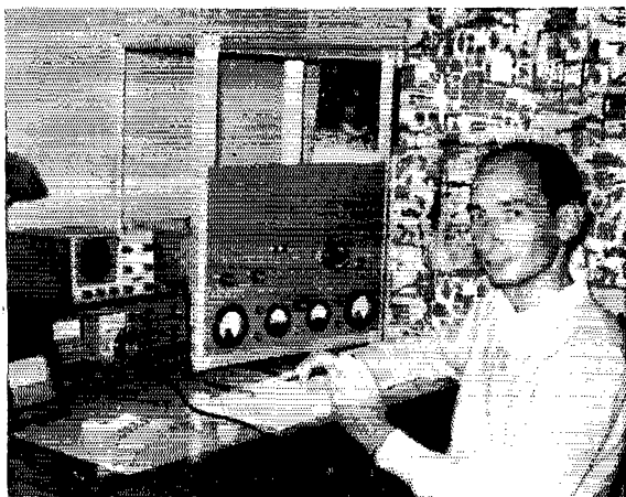
This is one of the most popular DX men on 50 MHz., Michael Czysch, LU3DCA, Buenos Aires, Argentina. The Swan 350 feeds 14 MHz. to a mixer which in turn drives three 4CX250Bs in parallel, producing 500 watts output on six meters.
