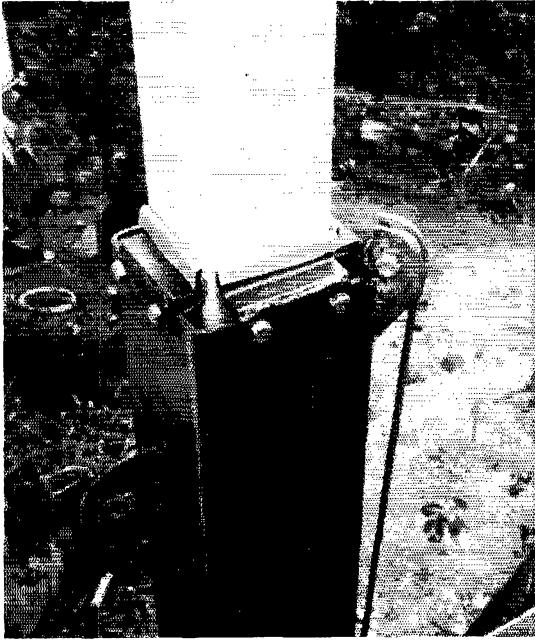
The pulley and guide arrangement. The large ear is for hoisting the mast into place.
