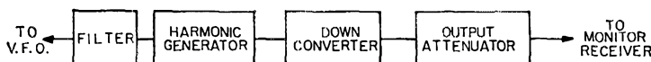
Fig. 1—Block diagram of the Chirp Magnifier. The unit should be built in a Minibox or other shielded enclosure to prevent direct radiation.
