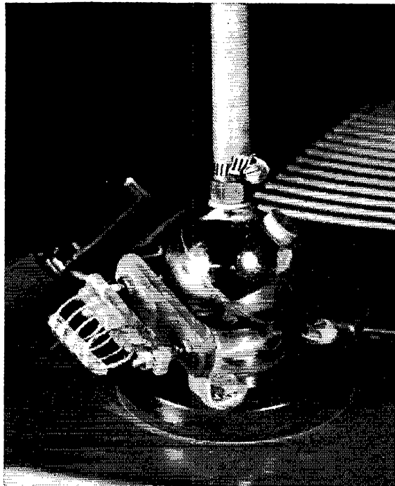
Shunt feed point, L_A . The matching coil shown is for 40 meters. RG-58/U coax, with a PL-259 plug and reducer, is connected to the body mount underneath the cowl.
