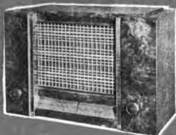
MOD. 871 MIDGET (CHASSIS 870) Supereterodina a 4 valvole
