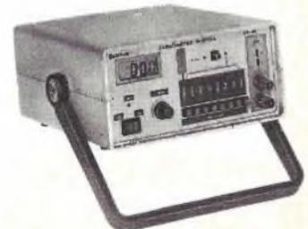
Instrumento preciso e prático, nas escalas de 200 pF, 2nF, 20 nF, 2  $\mu$ F, 20  $\mu$ F, 200  $\mu$ F, 2000  $\mu$ F, 20 mF.
