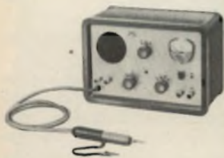
Signal Tracer tipo GM 7600
