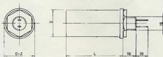
Per  $D = 35 \text{ mm}$   $\varnothing$  vite = 18 mm
