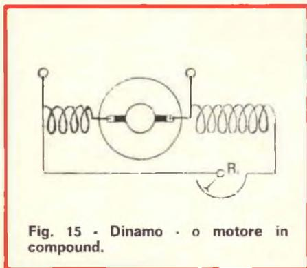
Fig. 15 - Dinamo - o motore in compound.
