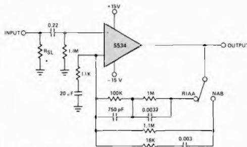
\*Select to provide specified transducer loading.
