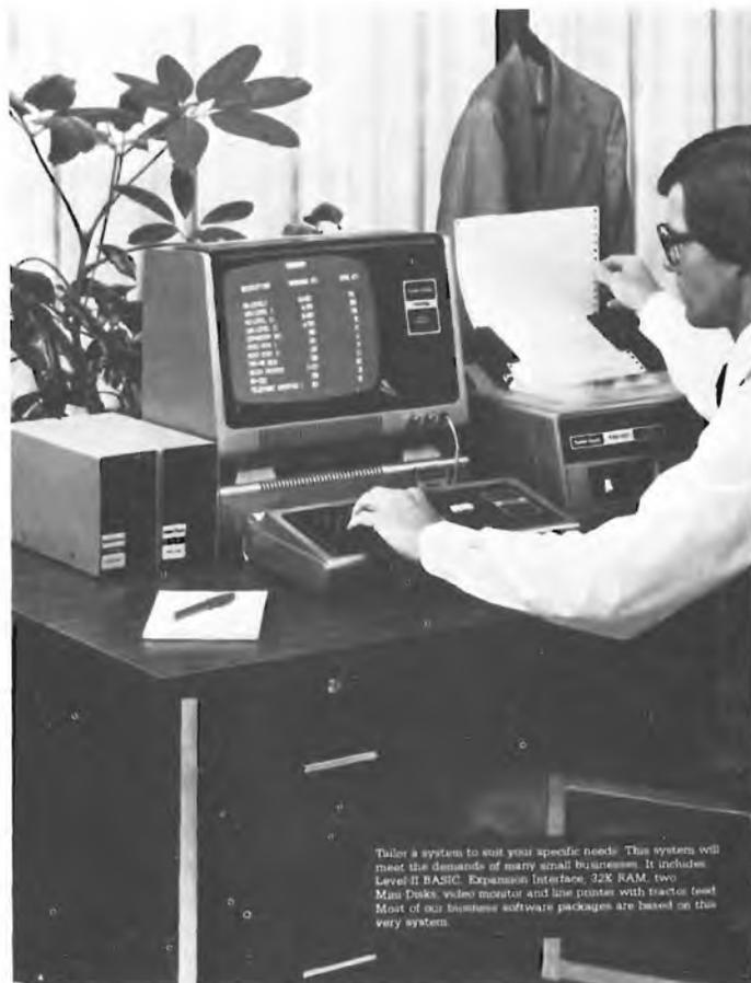
Tailor a system to suit your specific needs. This system will meet the demands of many small businesses. It includes Level II BASIC, Expansion Interface, 32K RAM, two Mini Disks, video monitor and line printer with tractor feed. Most of our business software packages are based on this very system.
