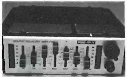
AMPLI-EQUALIZZATORE 25+25 W
