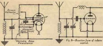
required for a mains variable mu is about 40 or 50 volts, thus it would be impracticable to supply this from batteries as in the battery arrangement of the variable mu. The easiest method of obtaining this voltage is to use automatic grid bias, by connecting a resistance between the high tension negative and the cathode of the variable mu The anode current of the valve passes through this resistance and a voltage drop is set up across it, making the
