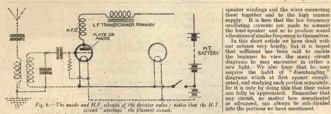
positive through the H.F. choke and L.F. transformer. It will be noticed that the high tension and filament circuits overlap to a certain extent, since one pole of both H.T. and L.T. batteries are connected together and to one side of the valve filament. The complete high tension circuit is often still further divided and we speak of the
