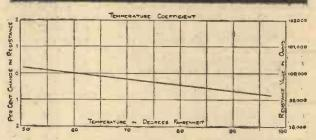
For every one degree centigrade rise in temperature the change in resistance value of a Qubilier resistance is only .04%. small effect of this change in the resistance value under normal working conditions is emphasised by the curve shown herewith, the right-hand scale of which gives the actual resistance values of a 100,000 ohm resistance at various temperatures; while the lefthand scale gives the average percentage changes.
