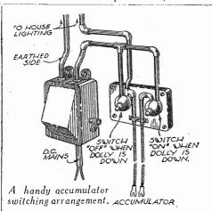
is inverted to enable the dollys to be raised or lowered together, thus facilitating a bar connector to absolutely ensure that accumulator is not shorted.—W. Jones (Smethwick).
