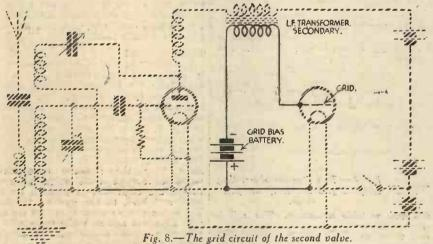
close to that in the grid circuit and so the magnetic fields of both "overlap." As a result high frequency current flows from one to the other just as it passes from the aerial to the grid coil. The amount of current which may pass back from the anode to the grid circuit is governed by the capacity of the reaction condenser and, therefore, by varying this the degree of feed-back (or reaction) can be controlled by the operator.
