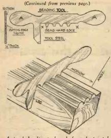
A simple beading tool made from sheet metal.
