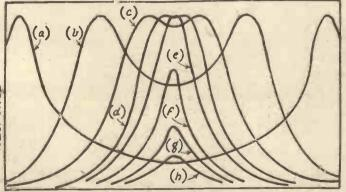
FREQUENCY maximum selectivity combined Fig. 1.-Resonance curves of a coupled circuit with various degrees of coupling.
