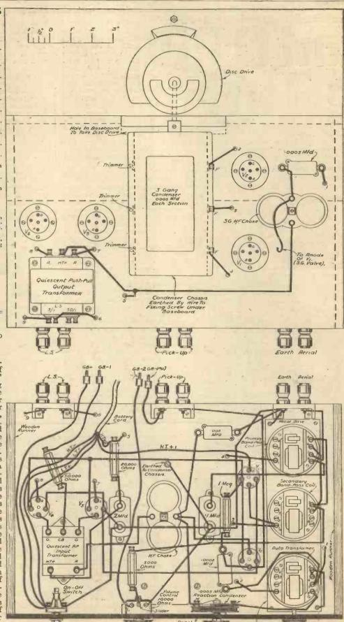
Top and sub-baseboard wiring of the Ferrocart Q.P.-P. Hi-mag Three.
