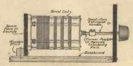
and removed the bakelite knob from the top. Then by boring a hole in the front panel and attaching a short-wave extension handle to the condenser spindle, I was able to re-attach the knob on to the extension handle, so that the selectivity could be controlled from the panel. This arrangement also helps to eliminate hand-capacity, when tuning in some of the weaker foreigners.
