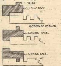
the slot cut, and you have a second guiding face which will keep the pitch of the slots constant. Another idea is to use two or three hacksaw blades in the frame at once.
