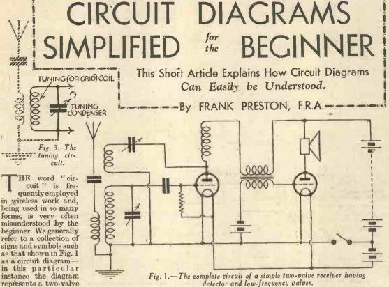
of a condenser just as easily as it flows through a length of wire. Without stopping to consider the theory surrounding the functioning of the aerial circuit we will pass
