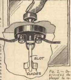
knob, and a new end piece, consisting of a small square block of ebonite, is screwed to the end of the plunger. To switch off the set the plunger is pressed, as indicated in Fig. 2, until the coin drops, thus breaking the circuit.—A. STEVENS (Rosherville).
