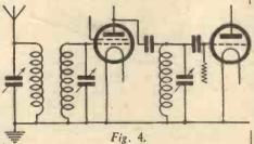
ferred to the second circuit. However, the gain in selectivity is such as to make it worth while. In this respect two coupled circuits differ from a single circuit, for as we have already seen none of the expedients which are normally used will
