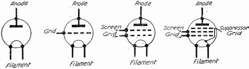
Fig. 1.—The evolution of the pentode valve.
