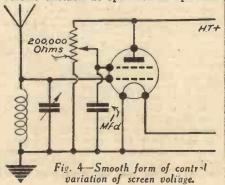
distortion. This form of volume control also varies the high-frequency amplification.
