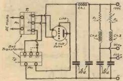
A cheap H.T. Eliminator using bell transformers.
