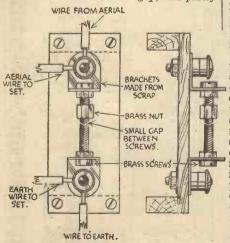
An aerial earthing device made from odds and ends, depends on the current be-
