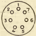
Fig. 1.—Showing the theoretical symbol for an indirectly heated H.F. pentode in conjunction with the corresponding value-holder connections. The value-holder is shown as seen from above.
