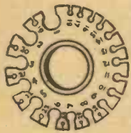
Fig. 1.—A circular gap-type wire gauge.
