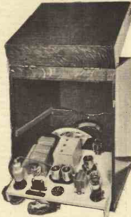
The receiver portion of the "Armada" in its cabinet. The mains unit shown on the right stands on the upper shelf.
