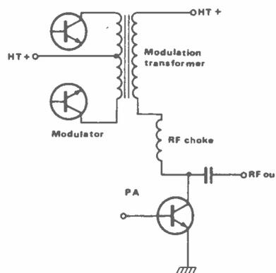
**Fig 1a** Amplitude modulation of a transistor PA using a modulation transformer
