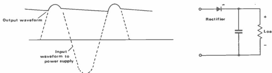
**Fig 7** Waveforms for a rectifier circuit using a reservoir capacitor C
