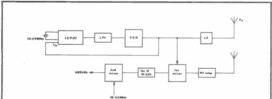
Fig 2 Block diagram of typical UK CB using LC7137
