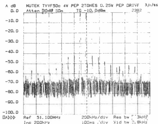
is way down at -71dB, the worst one being at -66dB at 200MHz which should not present any problem.
