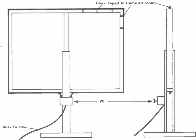
Fig 4 Details of the frame/co-ax arrangement
