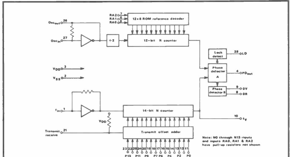
**Fig 7** Motorola MC145151 PLL chip
