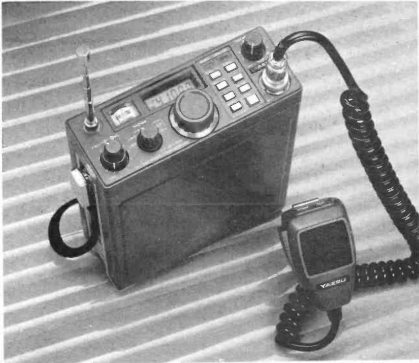
*Yaesu's FT290R is a portable multimode 144 MHz transceiver. Works well, with lots of facilities, puts out about 2.5 watts. Nice if you're a new Class B licence who likes a bit of fresh air!*
