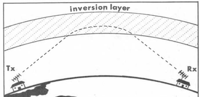
*Much closer to the earth than the D, E, F layers, the inversion layer will, in fact, refract VHF and UHF signals back to earth. Here, the waves are bent within the layer, rather than bounced off it.*
