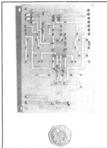
Typical amateur-made printed circuit board.
