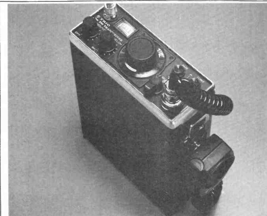
*Trio's TR2300 is a rather bulky 144 MHz hand-portable; 80 channels and about 1 watt output on FM, but there are easier ways of doing it these days and the basic design is a bit elderly. It produces lovely audio though.*
