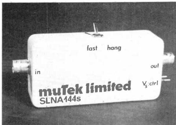
*muTek limited designs and manufactures high technology products for the keen radio amateur. Shown here is the SLNA144s 144MHz rf switched preamplifier — which we believe to be the best available. However that's only one of a wide range of products catering for interests from hf right through to the microwave amateur bands!*
