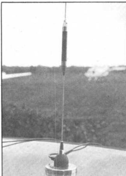
*Typical mag-mount mobile 70cm vertical antenna — note the loading coil partway up the rod.*
