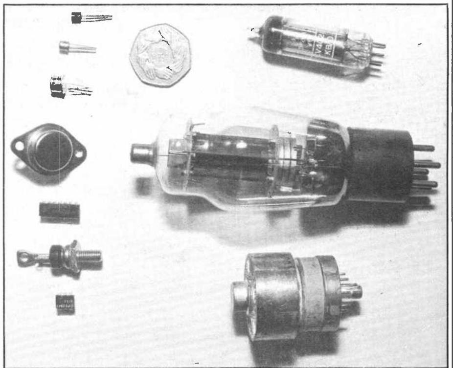
Selection of valves and semi-conductors.
