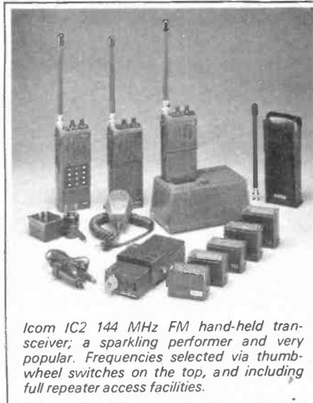
*Icom IC2 144 MHz FM hand-held transceiver; a sparkling performer and very popular. Frequencies selected via thumb-wheel switches on the top, and including full repeater access facilities.*
