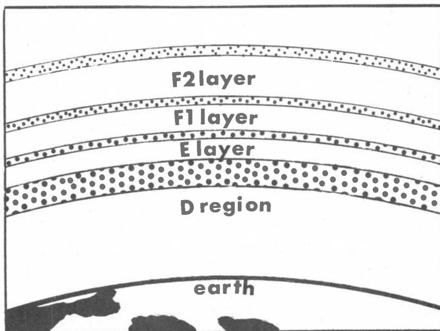
HF (High Frequency) signals can travel the world by bouncing off these layers. See the text for more details. VHF and microwave signals, however, won't. They'll pass straight through.
