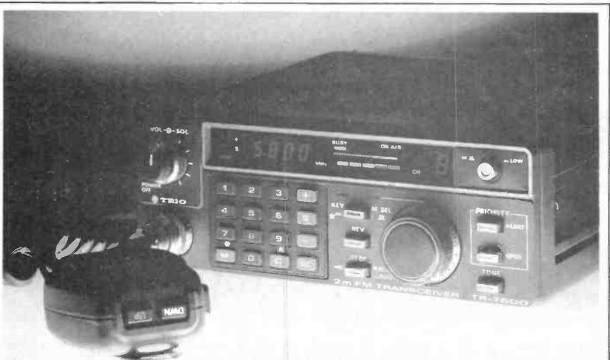
Trio TR7800 FM mobile 144 MHz rig, featuring selection of frequencies via a "keypad" and the ability to re-tune via switches on the microphone; an extremely good performer, with full repeater and simplex facilities in a compact box.
