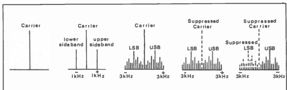
Diagrams illustrate the AM and FM wave forms, and how the single sideband radio wave is comprised. Note that SSB uses less of the spectrum in that only one of the bands (here, the upper sideband) is utilised to carry the message. Both the lower sideband and carrier are suppressed.
