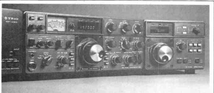
Trio TS830S — a typical upper-middle class HF SSB machine, developed from the very successful TS820. Very reliable and versatile; lots of facilities, excellent transmit strip but receiver lets the side down a bit . . . however, a pretty rig all in all.
