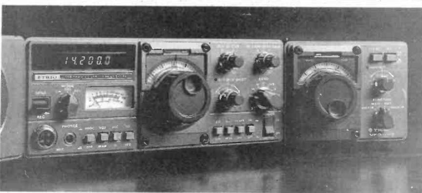
*Trio TS130S is a sort of transistorised variant of the TS530; the 130V is a lower-power version. Good middle-class radio for the newcomer.*
