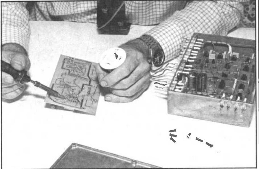
*Above: Soldering components on to a printed circuit board. Practice soldering and get it off to a tee before you work on the PCB. Below: Basic equipment needed in order to build your own radio, or carry out proper maintenance: screwdrivers, pliers and cutters, drills, soldering iron, and hacksaw.*
