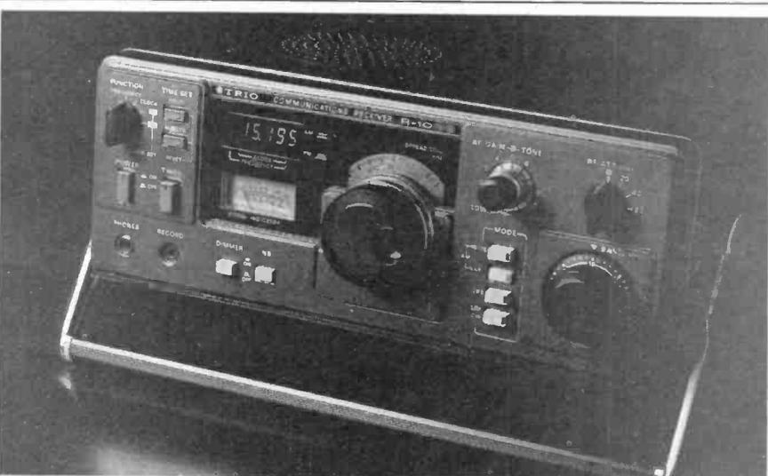
*Trio R1000 communications receiver. Extremely good for general HF listening, and full of useful features; a joy to operate and an excellent buy for the novice and expert alike. Covers all the HF spectrum with selection of tuneable 1 MHz bands and digital readout.*
