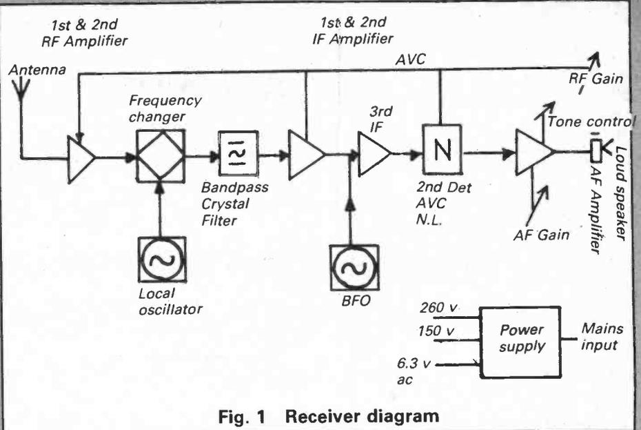
Fig. 1 Receiver diagram
