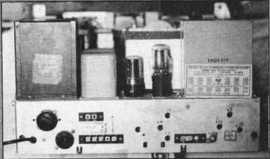
Above: The AR88 with its rear panel removed. Right: A simple antenna tuning unit for the frequency range 1.5MHz to 30MHz.
