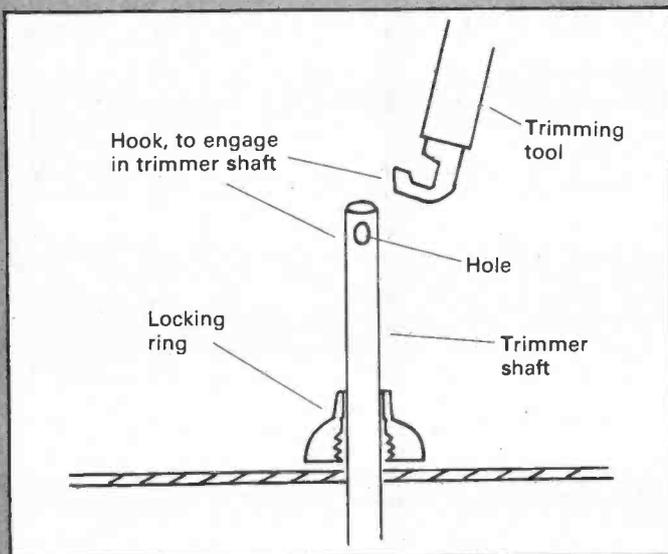
Above: This is a general guide to the control settings on AM, CW, SSB, and FM signals. There is, naturally, more information in the original manual - if you can obtain one. They are almost as valuable and rare as the equipment itself! Left: Details of the trimmer and the tool with which it can be adjusted. A well-kept AR88 should come supplied with two trimmer tools and an Allen key inside the cabinet.
