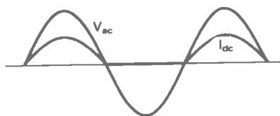
Half-wave rectifier and waveforms
