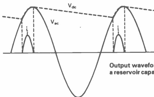
Output waveforms of rectifier circuit using a reservoir capacitor
