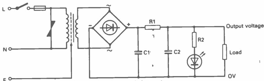
Practical power supply circuit (note the symbol for a bridge rectifier)
