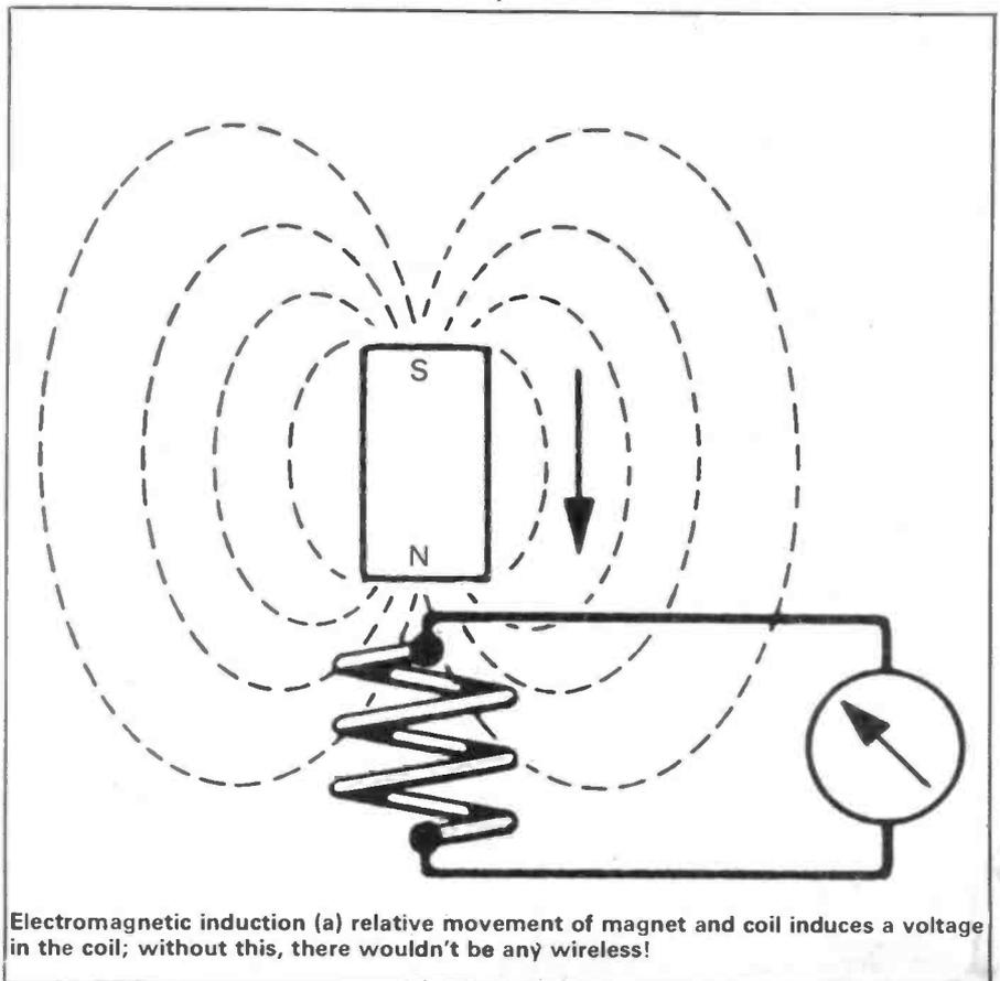
Electromagnetic induction (a) relative movement of magnet and coil induces a voltage in the coil; without this, there wouldn't be any wireless!
