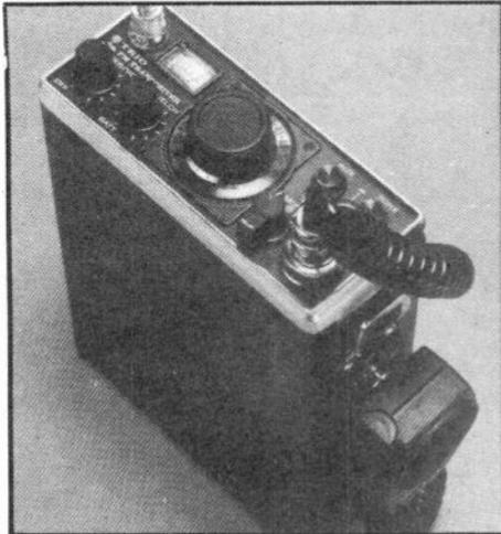
*This is Trio's 144MHz hand portable (TR2300) which has 80 channels and around one watt output on FM. Good audio sound.*
