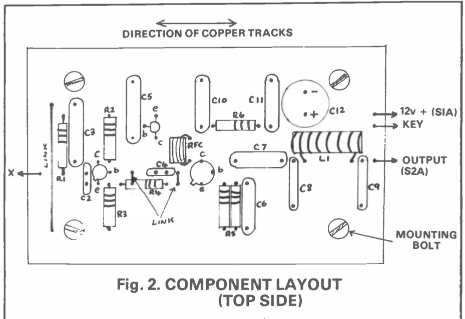
Fig. 2. COMPONENT LAYOUT (TOP SIDE)
