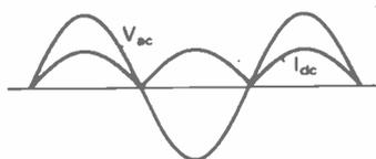
Full-wave rectifier and waveforms
