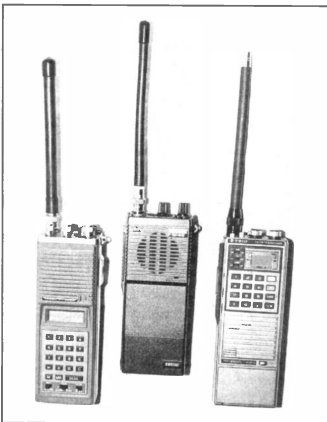
All three hand-helds look neat in their non-reflective cases, and short but businesslike antennae. From left to right are the Yaesu FT-208R, Icom IC-2E, and Trio TR-2500. Trio and Icom batteries have roughly the same capacity, while the Yaesu's battery is slightly larger. Current drain on the Trio was relatively high, with squelch on
