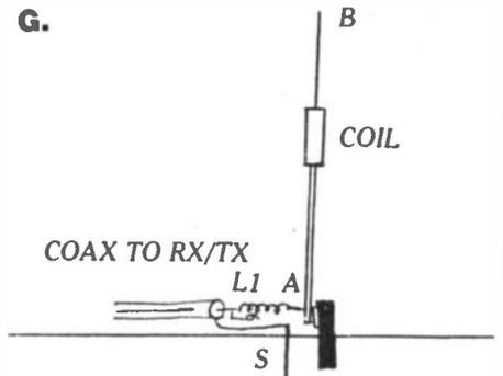
CENTRE: Front loaded vertical aerial from A to loading coil is 20' dural tube (length not critical). Coil should be wound on as greater diameter forms as practical with as thick wire as possible. From coil to B is 9' to 12' dural tube or tank whip. L1 variable induction (roller coil).
