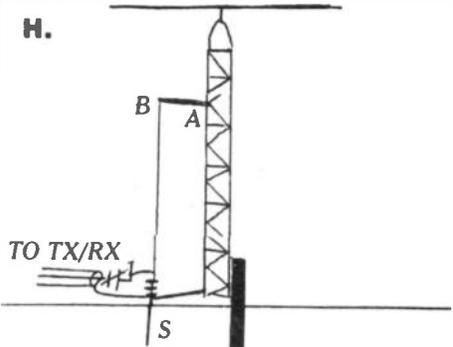
Gamma match feed of earthed tower. Correct impedance obtained by moving point A up and down tower, and by making A to B longer or shorter.
