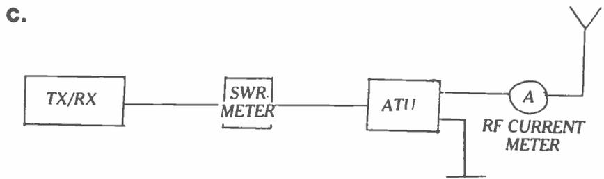
A method of connecting rig to end fed, current fed or other low impedance fed aerial. The SWR meter ensures a good match between rig and ATV. With such aerials (e.g. 132' wire) the object is to get as much RF current as possible indicated in the RF ammeter. The reading on the ammeter will depend upon aerial length and earth efficiency. Add radials or earth spikes until a greater reading cannot be obtained.
