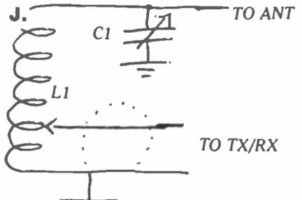
L1 35 turns 16 SUG 2" former 4" long tapped 5 turns up C1 500pf broadcast type variable.
