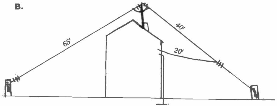
A method of fabricating an inverted vee aerial (quarter wave) over a house. This does work and can be fitted into small gardens. It is, however, much inferior to the half wave. If open to an upstairs shack the length of conductor to earth affects performance and increases noise pick up (live should be insulated from all anchor points). (The aerial can be bent round to suit individual site).
