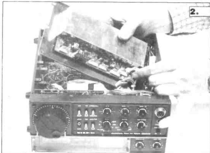
**2.** Remove power supply assembly by removing fixing screws. Disconnect multipole connector and put assembly to one side.
