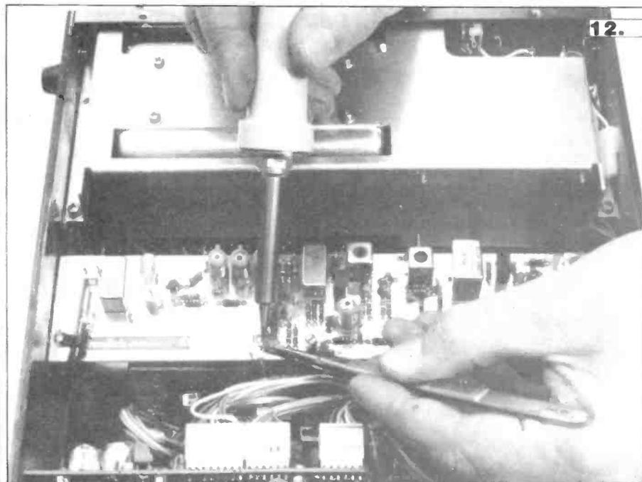
**12.** Fix Mutek board with two screws provided to existing (unused) diecast lugs, and as per detailed, fixing solder colour coded cables to the appropriate pins. Replace both covers and get out amongst the dx!
