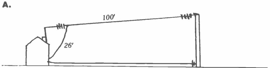
A method of turning a quarter wave inverted L aerial against a counterpoise. The counterpoise is a quarter wave length of insulated wire running about one foot above ground level. One end is connected directly to the rig on ATV and the other end disconnected. Improved performance can be obtained by using several similar radials all connected together at one end and laid out like spokes of a wheel. (If radials are used the equipment should also be earthed for safety purposes).
