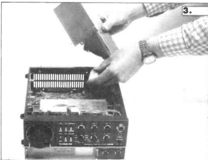
**3.** Remove synthesiser assembly. Do NOT forget fixing screw located through main pcb. Note positions of connectors and remove. Lift assembly clear.
