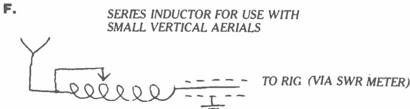
If a series inductor is used, the mobile whip should be adjusted to resonate on the highest frequency required. By increasing the number of turns in the series inductor (which can be in the shack) the frequency of the aerial system is lowered. Series Inductor can be ex government roller coaster type or made up of 16 SUG wire space wound 25 turns 1" to 2" diameter. Adjust for maximum aerial current and minimum SWR.
