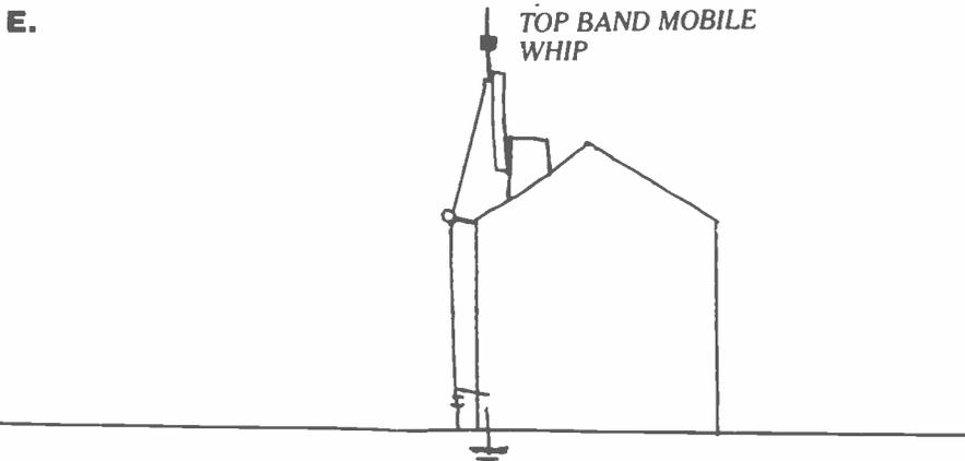
An old or redundant mobile whip can be used by connecting its base to an insulated (non metallic) pole attached to chimney etc. The base is connected to wire down lead and taken via a stand off insulator to the shack. The whip and the downhead will act as the aerial, but the conductor below the loading coil does the work. Such a system can be turned by using a series tuned ATV or a series inductor.
