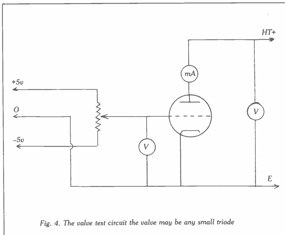
Fig. 4. The valve test circuit the valve may be any small triode
