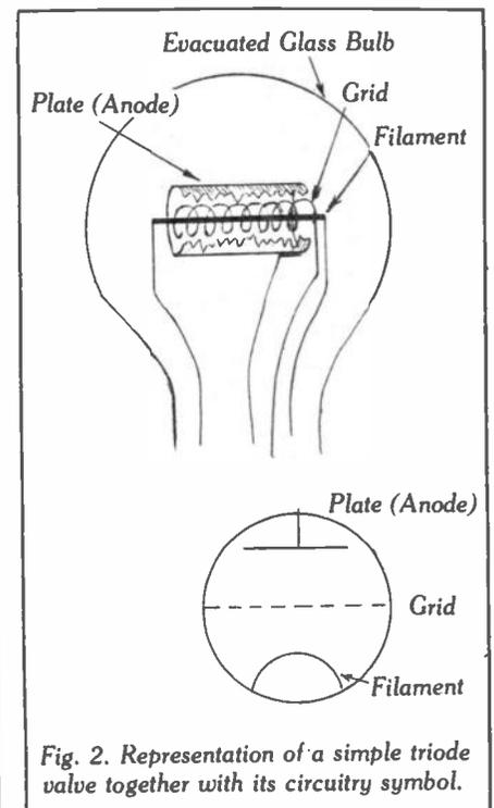
Fig. 2. Representation of a simple triode valve together with its circuitry symbol.
