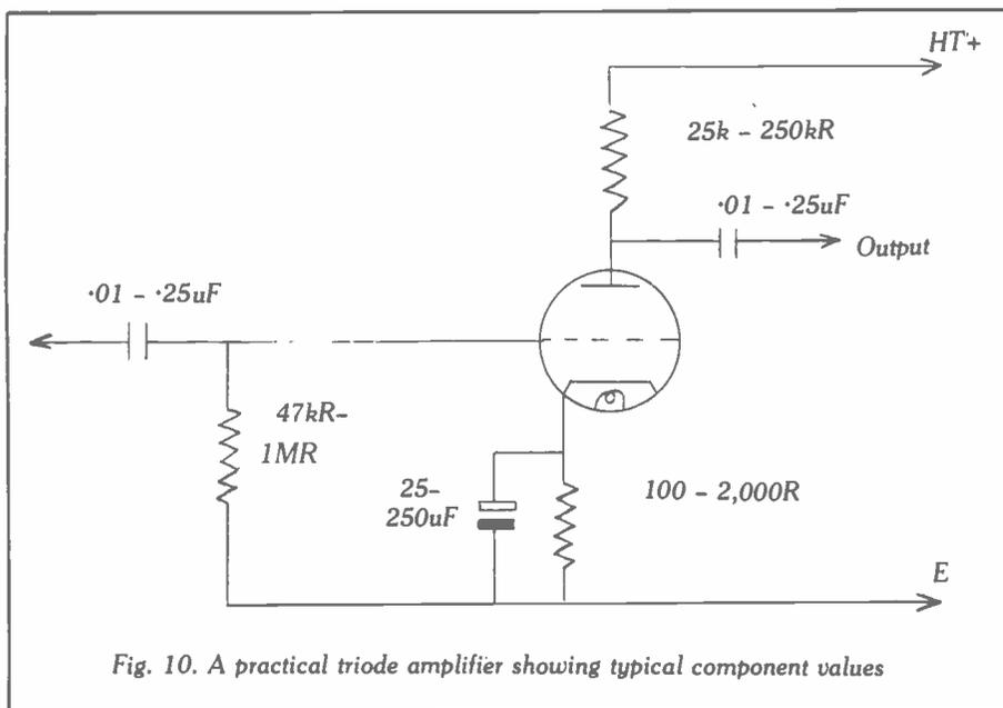
Fig. 10. A practical triode amplifier showing typical component values
