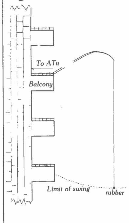
It could also be made up from bamboo with thick wire taped along its length. For single band operation the chimney vertical is best cut to a quarter wavelength at the working frequency and there should be a piece of wire of identical length to run around the edges of the room or under the carpet to serve as the ground plane. Any other metal piping or heating radiators can also serve as additional earthing to supplement the single 'radial'.
