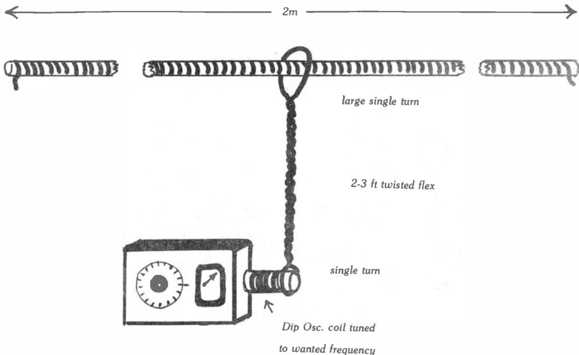
Setting up the  $\frac{1}{2}$  coil with a Dip Oscillator
