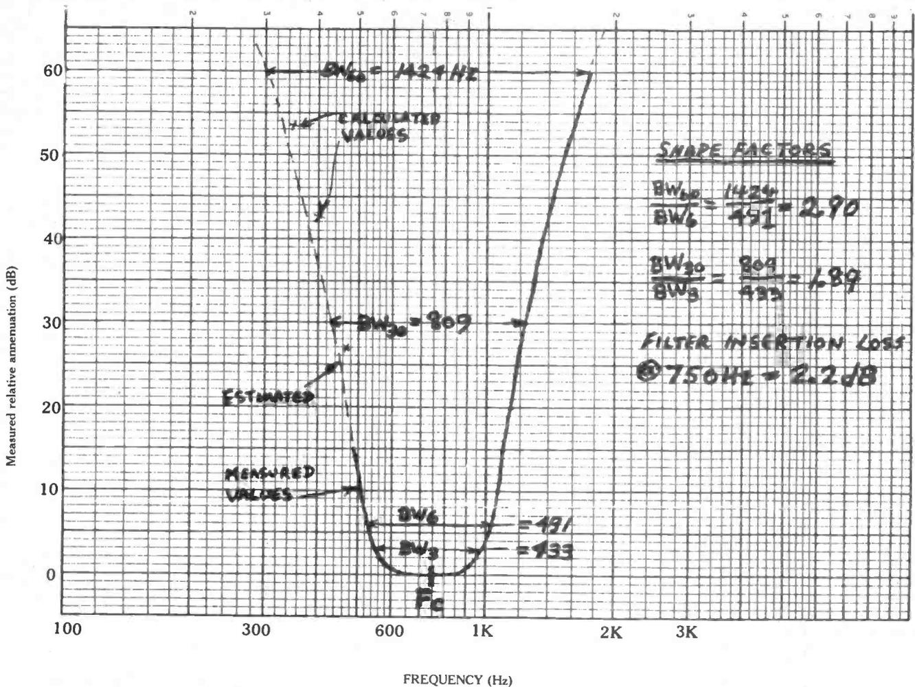
Measured relative attenuation vs. frequency for a single stack (C-O-J) CW filter W3NQN 26MAR83
