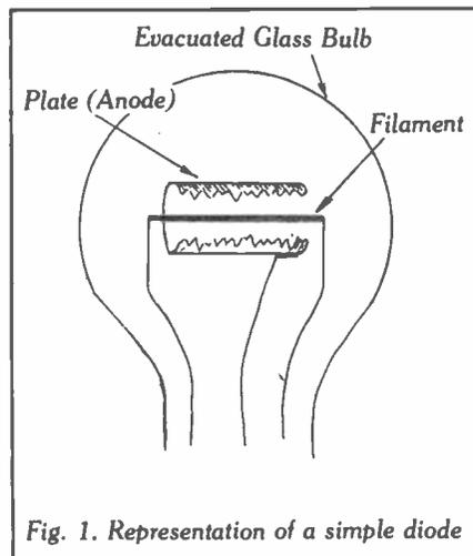
Fig. 1. Representation of a simple diode
