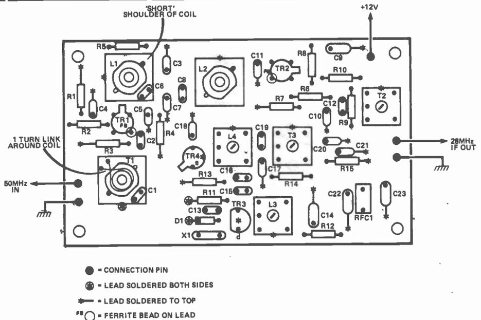
To ensure stability, the converter has been designed onto a double sided PCB, with the upper foil used as a ground plane for the earth connections. All components mount on this side of the board, and in this way are screened from the tracks carrying signals on the underside. Additional screening cans are used on the topside around all coils and transformers.
