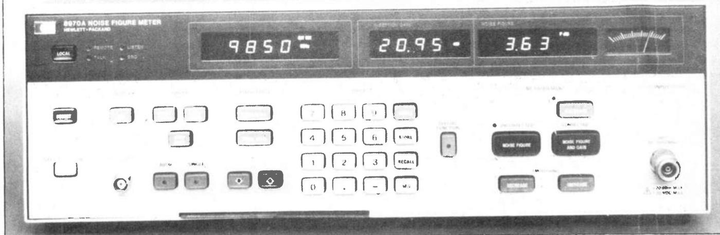
Above: the Hewlett Packard 8970A noise figure meter, used by Angus McKenzie for last month's review of preamps, converters and transverters.
