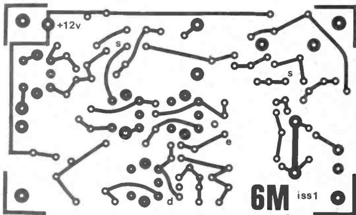
6. Insert the solder TR1 and TR2. The tab should point in the direction shown, and a miniature ferrite bead is placed over each gate 1 lead before pushing into the holes. The transistor then rests on the bead. These MOSFETS are protected against static charges, so no unusual precautions need be taken, although you should ensure that your soldering iron is earthed, or that it is an isolated type.
