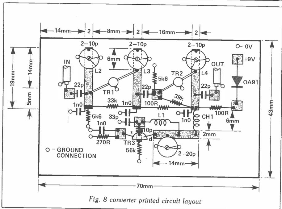
Fig. 8 converter printed circuit layout
