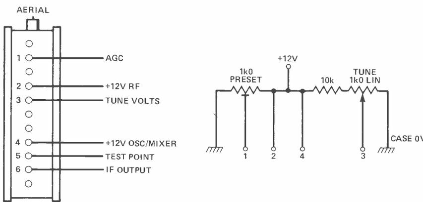
Fig. 5: ELC1043 pin connections and wiring
