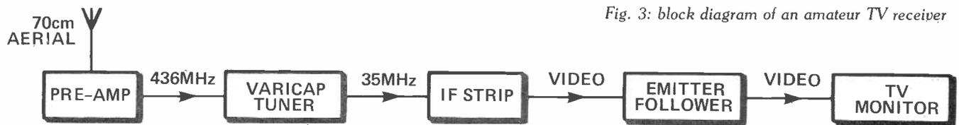
Fig. 3: block diagram of an amateur TV receiver
