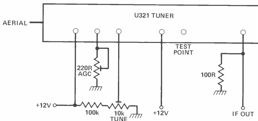
Fig. 6: U321 wiring for 70cm operation
