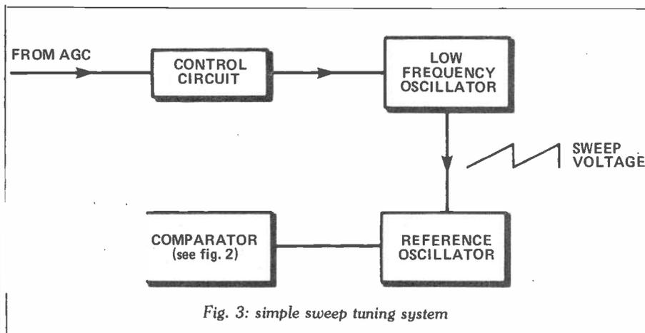
Fig 3: simple sweep tuning system
