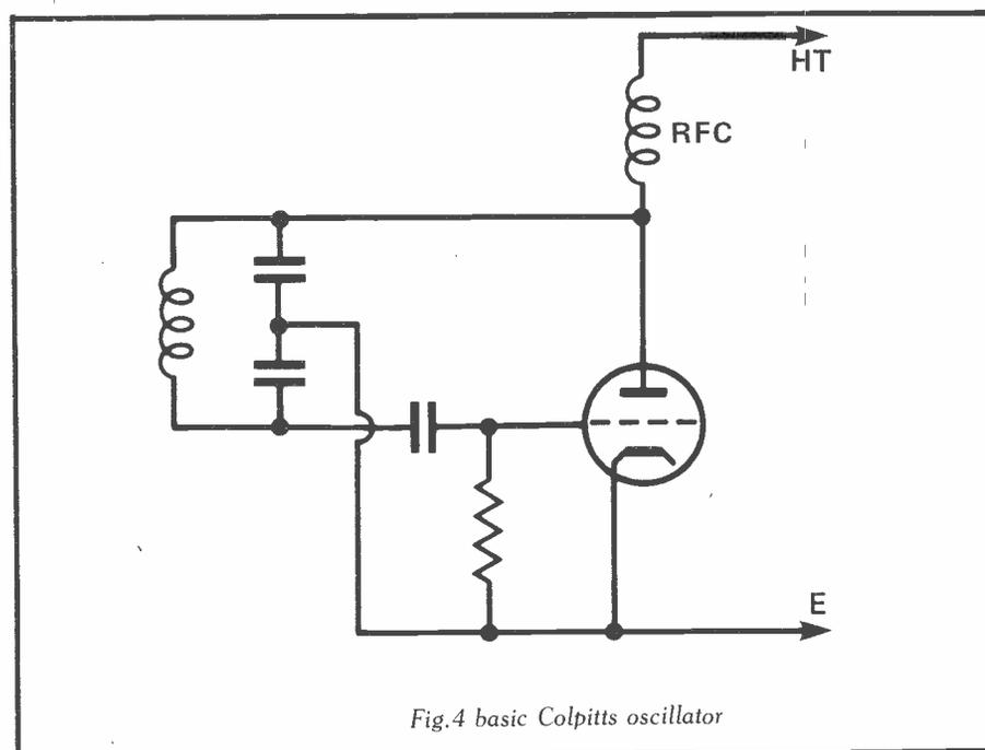
Fig.4 basic Colpitts oscillator
