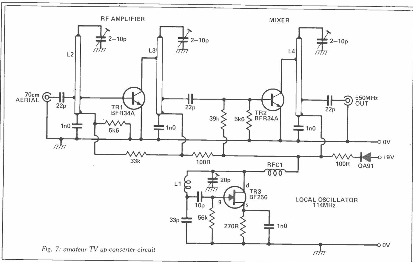
Fig. 7: amateur TV up-converter circuit
