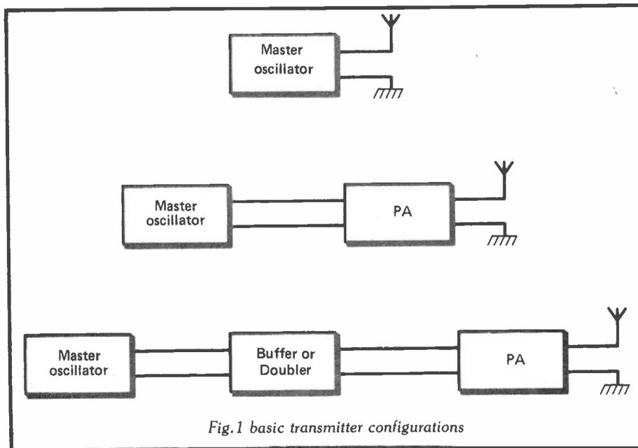
Fig.1 basic transmitter configurations
