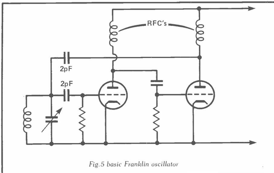
Fig.5 basic Franklin oscillator
