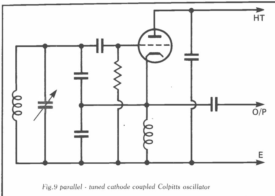
Fig.9 parallel - tuned cathode coupled Colpitts oscillator
