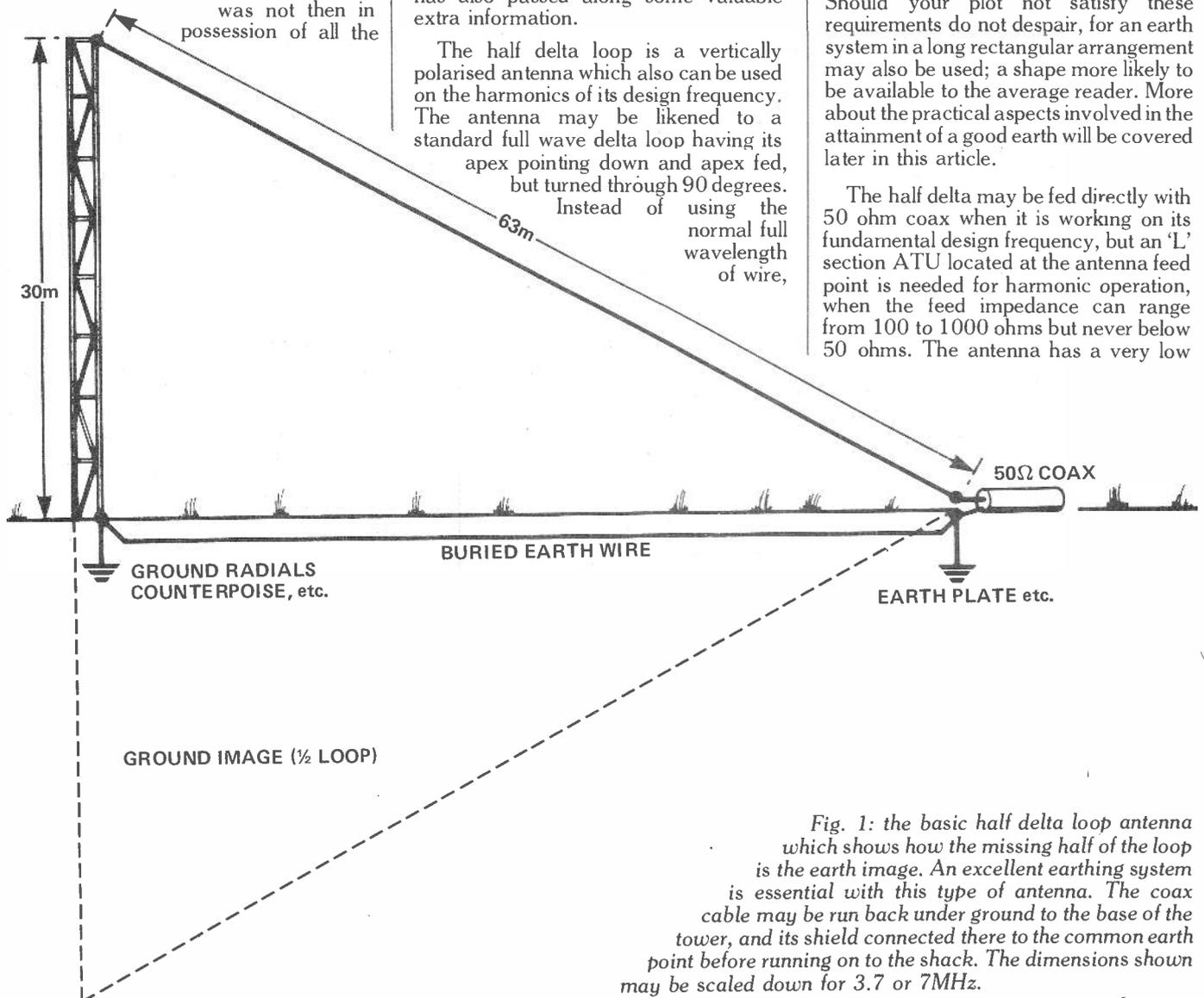
Fig. 1: the basic half delta loop antenna which shows how the missing half of the loop is the earth image. An excellent earthing system is essential with this type of antenna. The coax cable may be run back under ground to the base of the tower, and its shield connected there to the common earth point before running on to the shack. The dimensions shown may be scaled down for 3.7 or 7MHz.
