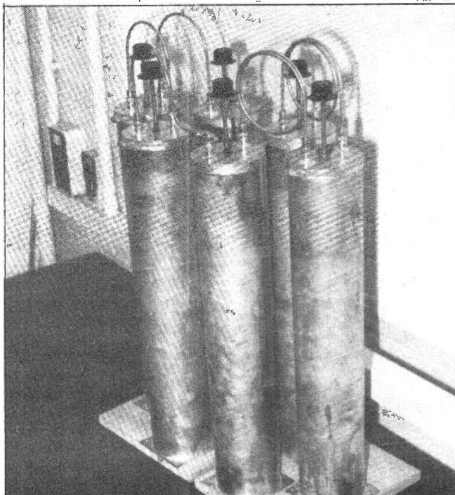
Six filters connected to form the receive/transmit aerial combiner.
