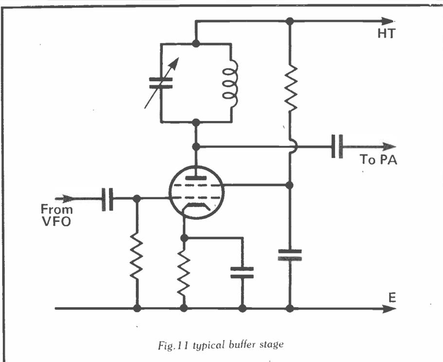
Fig. 11 typical buffer stage
