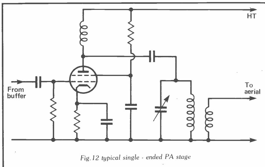
Fig. 12 typical single-ended PA stage
