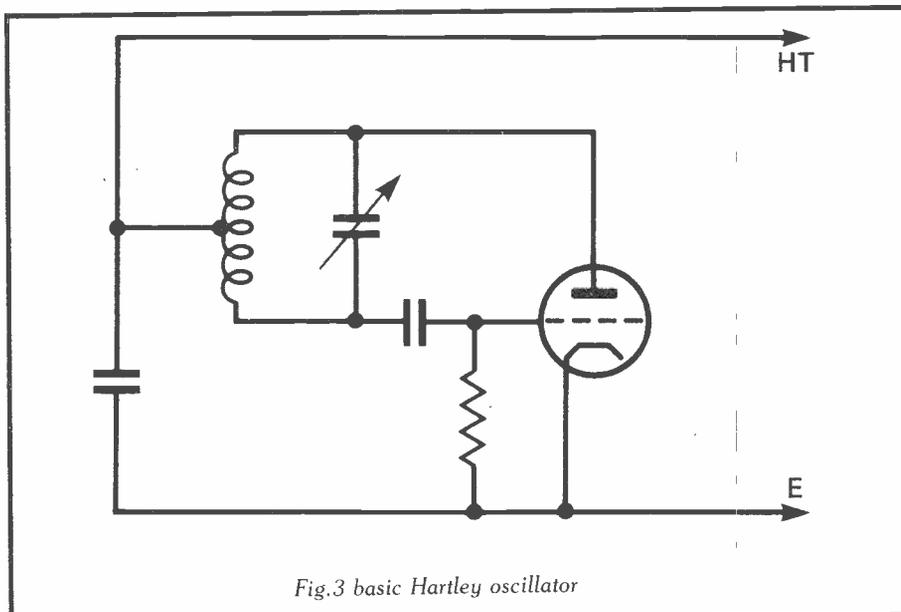
Fig.3 basic Hartley oscillator
