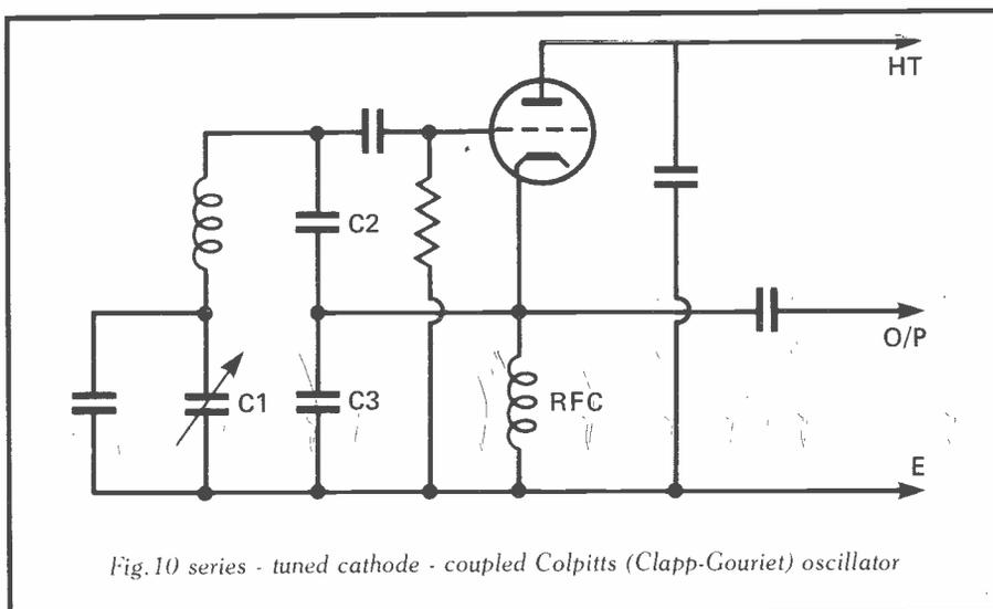
Fig.10 series - tuned cathode - coupled Colpitts (Clapp-Gouriet) oscillator
