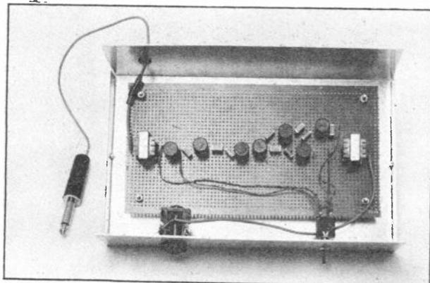
View of the filter constructed on Veroboard. Keeping the input and output sections well separated reduces leakage past the filter.
