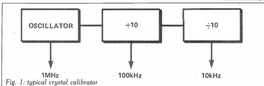
Fig. 1: typical crystal calibrator
