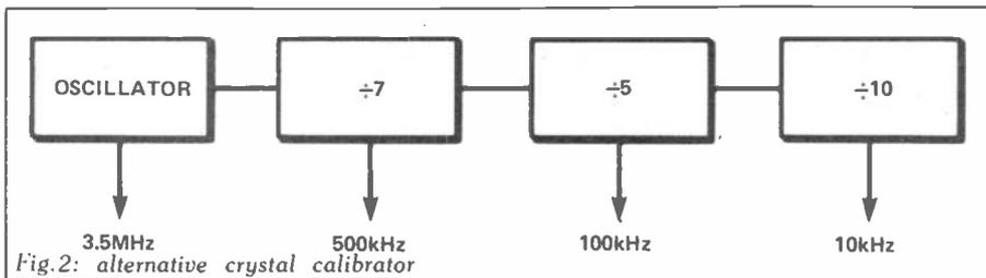
Fig.2: alternative crystal calibrator
