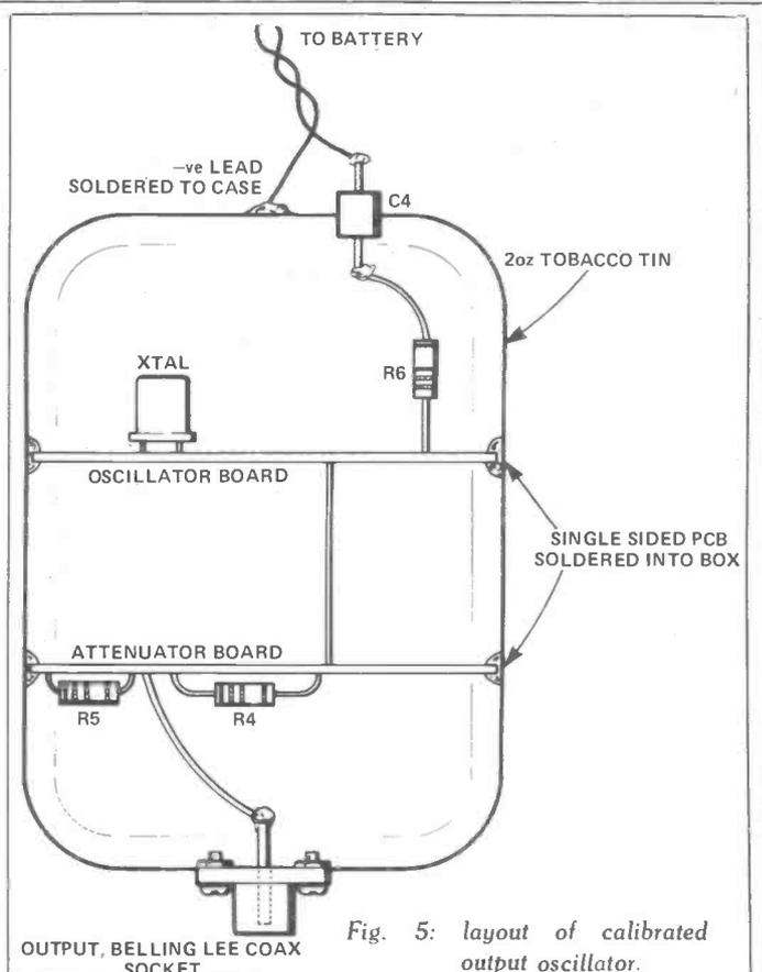
Fig. 5: layout of calibrated output oscillator.
