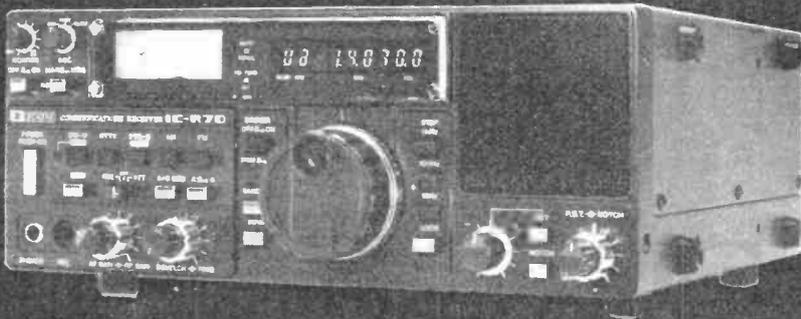
The R70 covers all modes (when the FM option is included), and uses 2CPU-driven VFOs for split frequency working, and has 3 IF frequencies: 70MHz, 9MHz and 455KHz, and a dynamic range of 100dB. It has a built-in mains supply. Other features include input switchability through a pre-amplifier, direct or via an attenuator, selectable tuning steps of 1KHz, 100Hz or 10Hz, adjustable IF bandwidth in 3 steps (455KHz). Noise limiter, switchable
