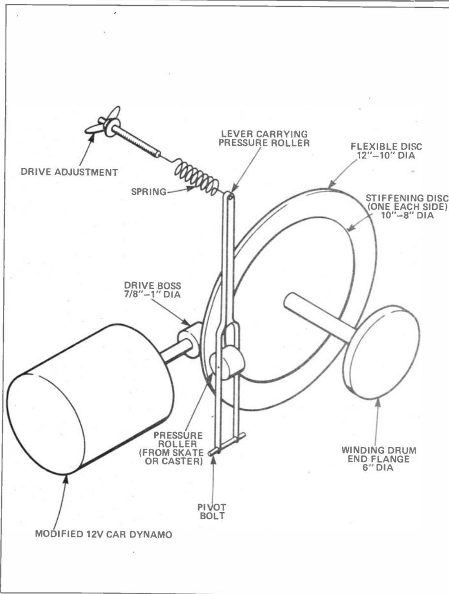
Fig. 2: an ultra basic reduction drive
