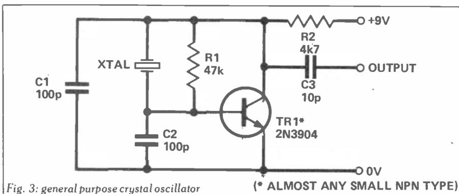
Fig. 3: general purpose crystal oscillator
