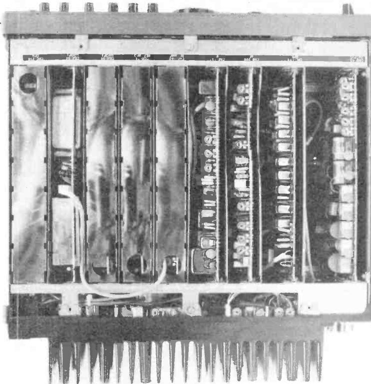
The JST-100 is built on a mother and daughter board system, making maintenance much easier than usual. Bottom: the sockets on the back panel, going from left to right, are for DC power, accessory, coupler, memory, key, speaker, line out, IF out, RX ant. The main antenna socket is shown top right.
