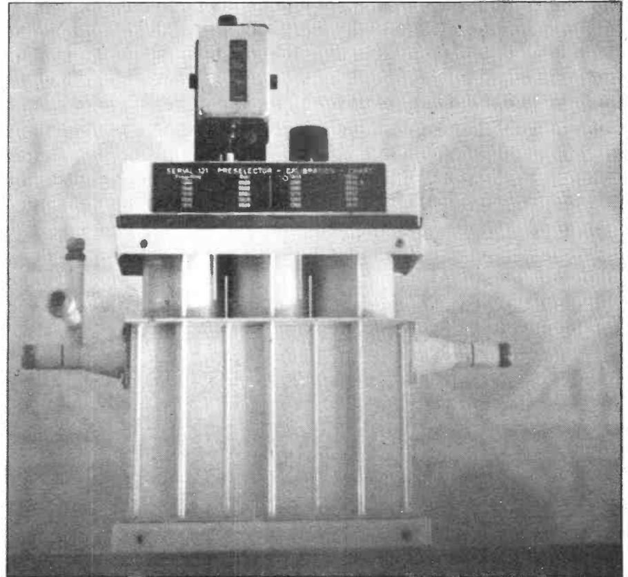
Tunable bandpass filter covering 1250-1350MHz (bandwidth 5 to 8MHz), obtained at a Leicester rally.
