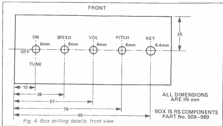
Fig. 4: Box drilling details: front view
