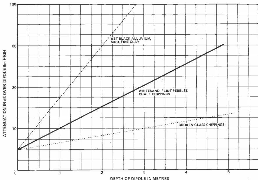
Fig. C Graph displaying the attenuation at different depths and in different surrounding media. It will be noticed that even at ground level there will be attenuation.
