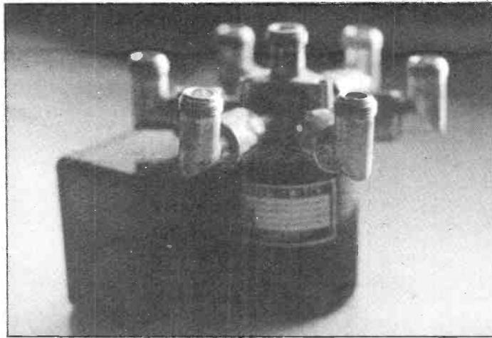
Surplus six-way aerial switch: the seven type N sockets are a single casting! Operated by a 24V solenoid, to which I have added a homebrew control panel.
