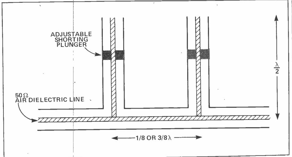
Two stub tuner: schematic diagram. As the lengths of the stubs are altered, different values of inductive or capacitive susceptance are added to the 50 ohm line section.
