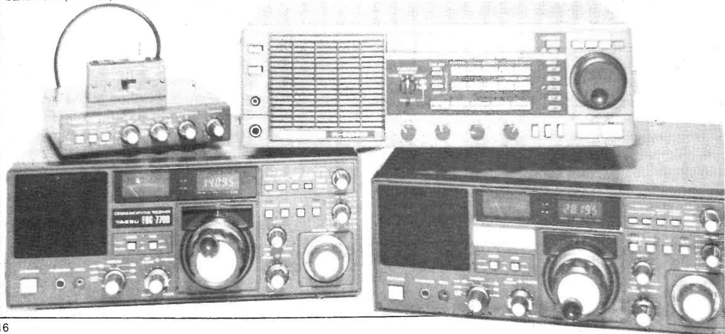
the receiver is muted allowing it to be used with a transmitter. An extension speaker can be interconnected with a 3.5mm jack socket. The set can be used either with normal AC mains or 13v DC, a separate socket being provided for the latter. An accessory socket provides 11v DC, the AGC line, mute output and ground.
