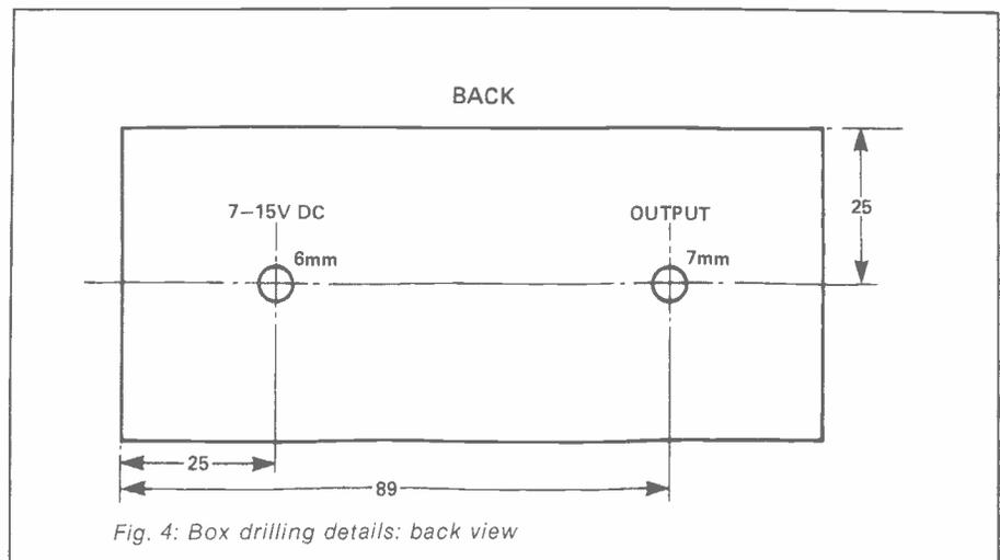
Fig. 4: Box drilling details: back view
