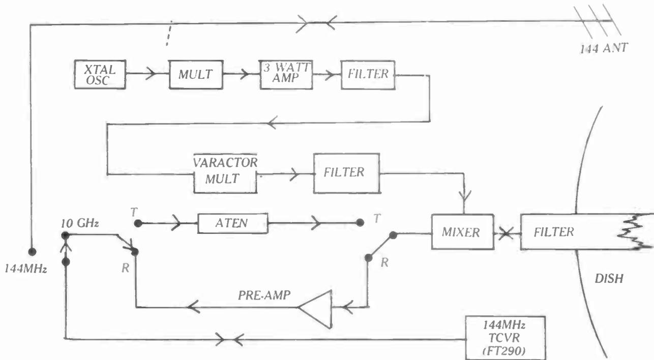
Block diagram of "narrowband SSB" system
