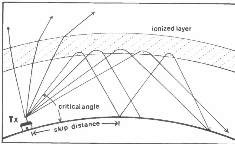
Left: What radio waves do when they reach an ionized reflecting layer. Receivers within the skip distance won't hear your signal, of course.
