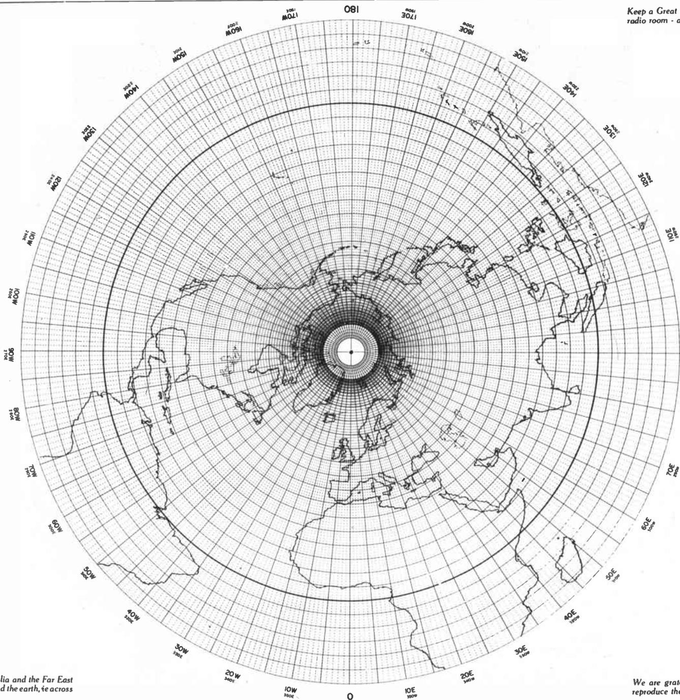
The Great Circle Map should be consulted along with the radiation pattern of your antenna for long distance DX work. Such a map is absolutely essential if you are planning a proper antenna installation. Remember, incidentally, that in the mornings, signals from (and to) Australia and the Far East can sometimes travel the other way round the earth, i.e. across South America.
