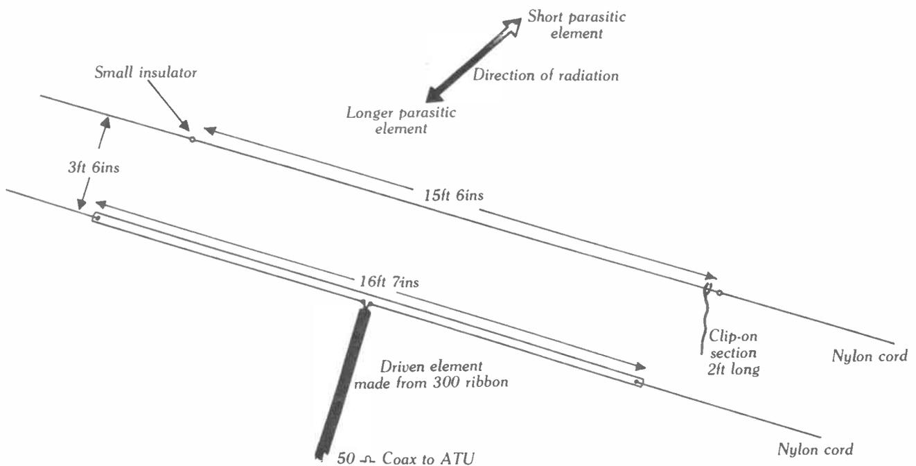
**Fig. 2. Constructional details of a two element indoor two-way beam for 28 MHz.**
