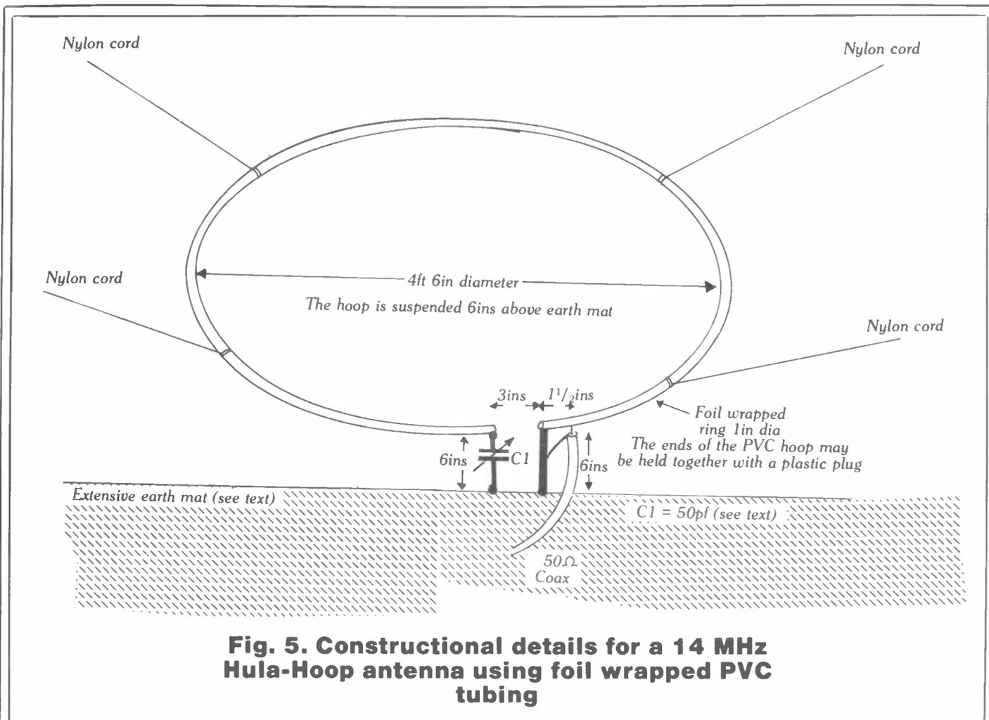
**Fig. 5. Constructional details for a 14 MHz Hula-Hoop antenna using foil wrapped PVC tubing**
