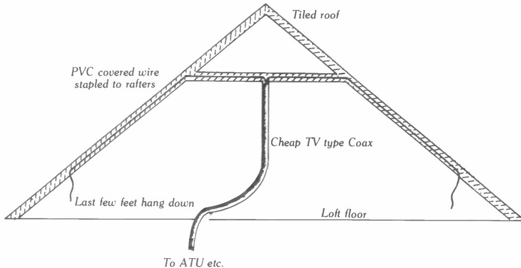
**Fig. 1. How the G4BSW Loft Dipole is arranged**
