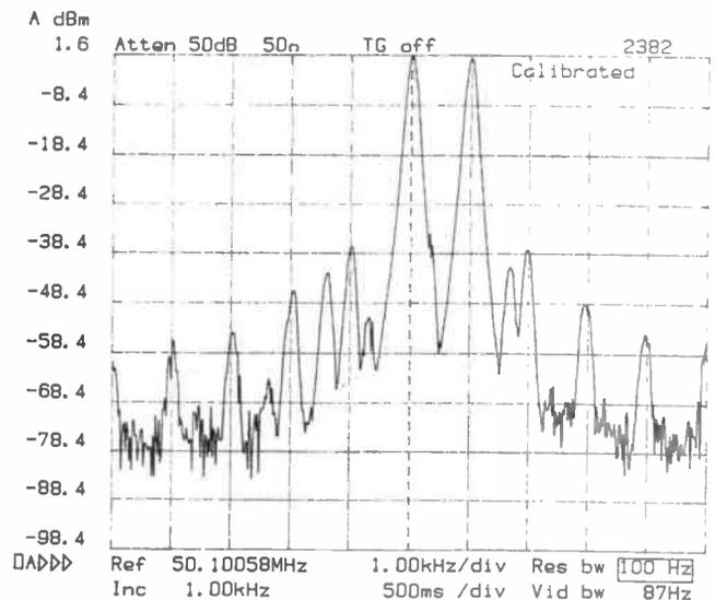
Two-tone test of TS670 on 50.1MHz at full power
