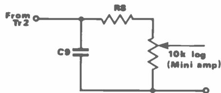
Fig 6 Input circuit to mini-amp
