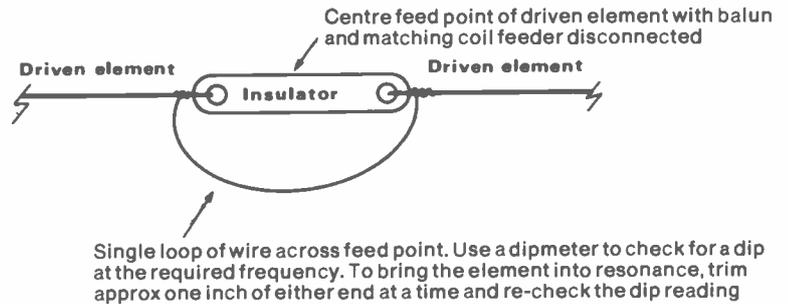
**Fig 3** Checking the driven element for resonance
