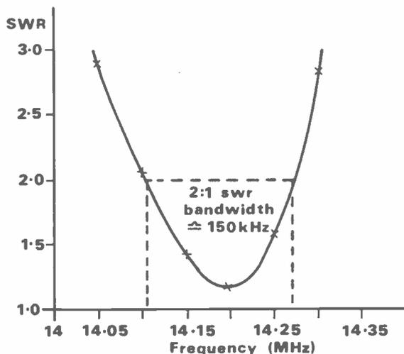
Fig 5 SWR v frequency plot for the author's prototype beam
