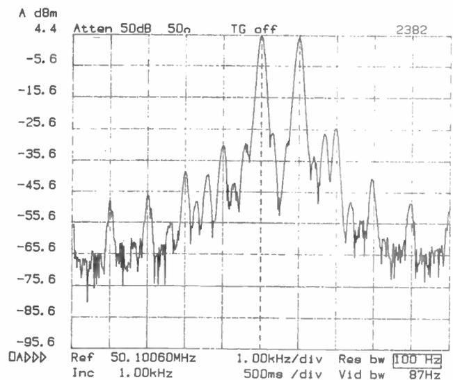
Complete transmitted response from mic socket input to RF carrier output, well below any ALC action showing filter response, alternate sideband and carrier rejections
