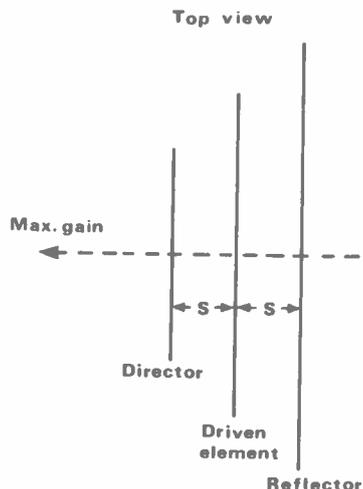
The spacing (S) is between  $0.1\lambda$  and  $0.15\lambda$ . Element lengths are worked out from the following formula:
