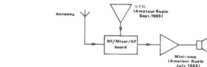
Fig 1 AR80m receiver block diagram
