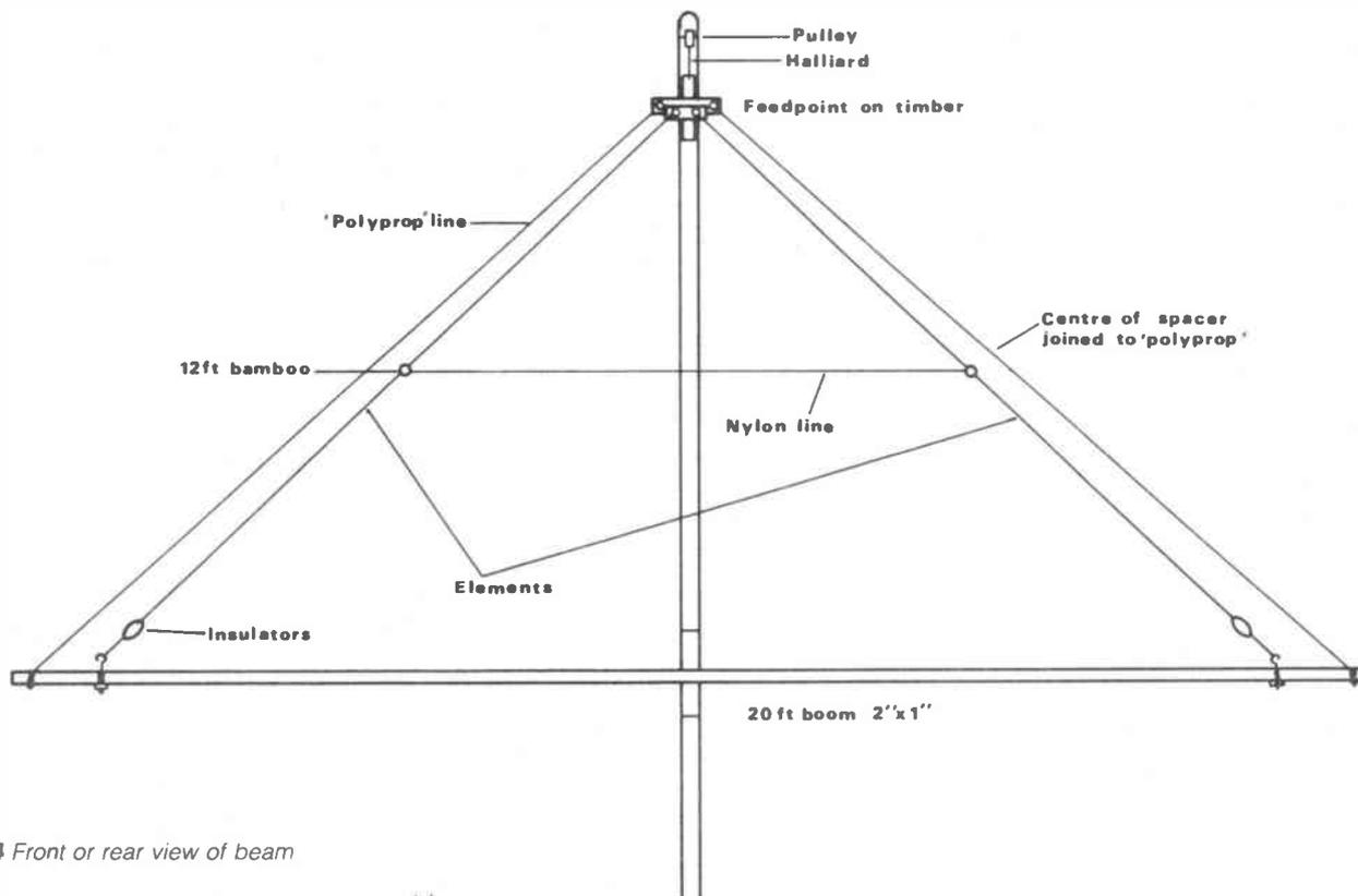
Fig 4 Front or rear view of beam
