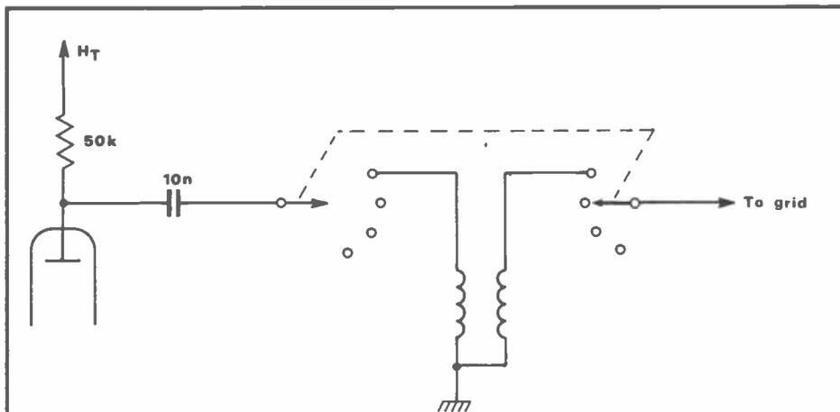
Fig 1 Common type of circuit for basic valve receivers
