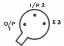
Fig 3 Underside view of ZN414
