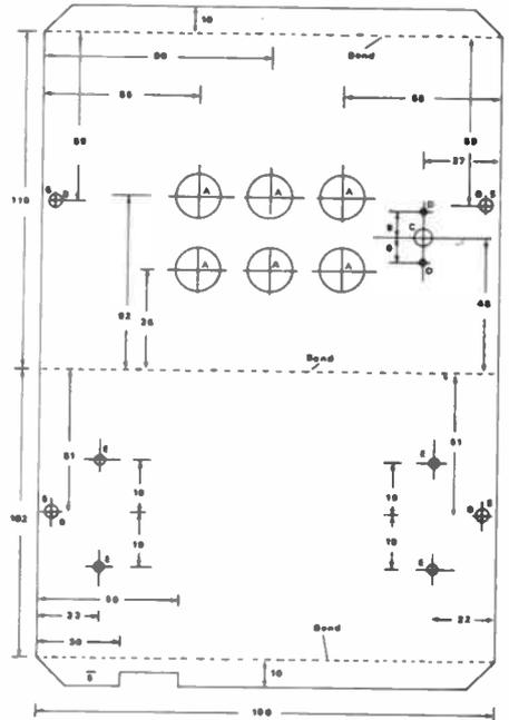
Fig 6 Dimensions of the back and bottom panels of the master oscillator box
