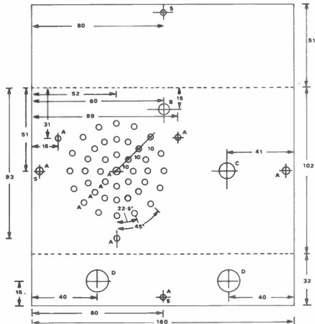
**Fig 9** Component layout for the 8 pin LM380 audio amplifier
