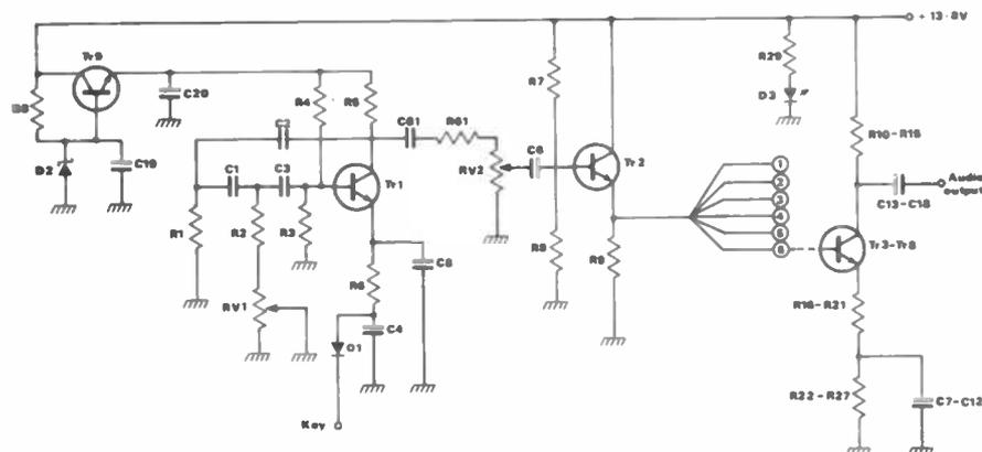
Fig 2 Full circuit diagram of master oscillator
