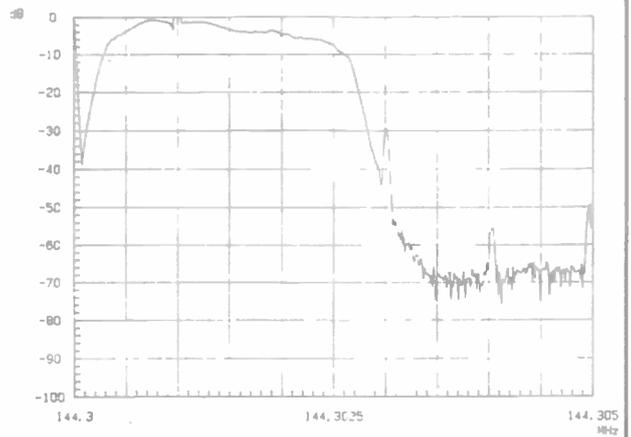
*IC275E USB two-tones 28W into ALC 700Hz/1 7kHz Resolution bandwidth 100Hz 2kHz per division*
