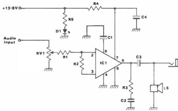
**Fig 8** Head end amplifier using 14 pin version of the LM380 IC
