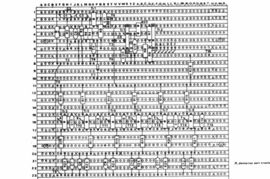
Fig 3 Component layout of master oscillator circuitry
