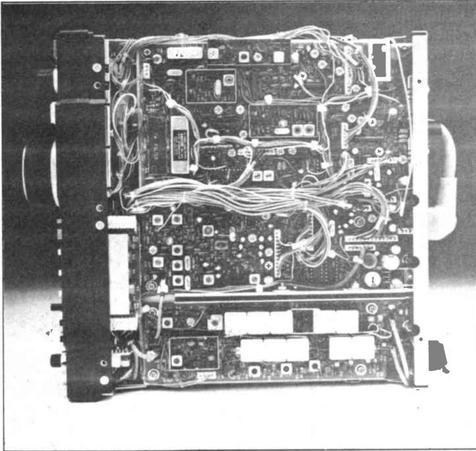
second mixer, a PC1037 double balanced IO, which mixes the signal down to the second IF at 455kHz. An FL65 2.4kHz ceramic ladder filter then follows, and after amplification the signal passes through to the product detector and audio stages.
