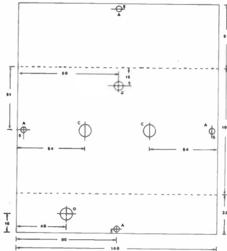
Fig 5 Dimensions of the front panel of the master oscillator
