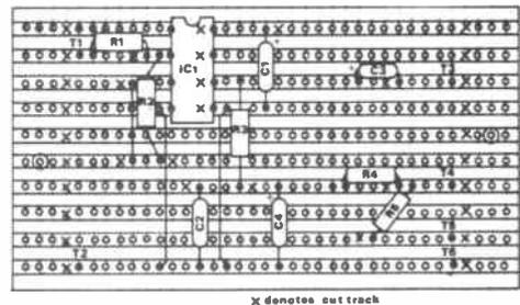
**Fig 10** Component layout for the 14 pin LM380 audio amplifier
