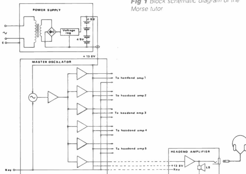
Fig 1 Block schematic diagram of the Morse tutor
