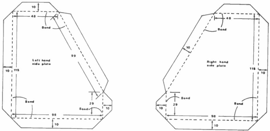
Fig 4 Dimensions of the two side panels
