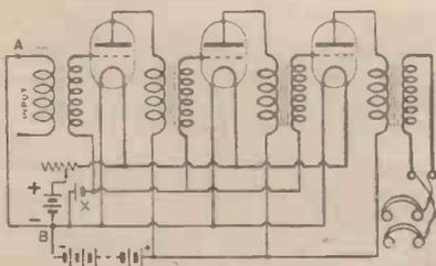
Fig. 2.—Connection Scheme of C Mark III Low-frequency Amplifier.
