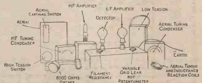
Photograph and Key Diagram of the Three-valve Receiving Set constructed by Mr. J. Seabrook, of the South London Wireless and Scientific Club.
