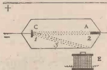
Fig. 3.—Diagram showing the Deflection of Cathode Rays by a Magnet.
