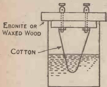
Fig. 4.—Damp-cotton Grid Leak.
