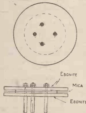
Fig. 9.—Design for 2-slot, “Plug-in” Type H.F. Transformer.
