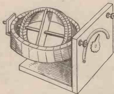
Fig 5.—The Variometer Complete.
