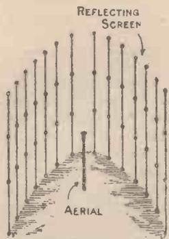
Fig. 1.—Diagram of the Parabolic Form of Transmitting Aerial System.
