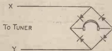
Fig. 1.—Circuit with Four Crystals.
