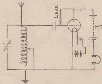
Fig. 10.—Another Grid-leak Connection Diagram.
