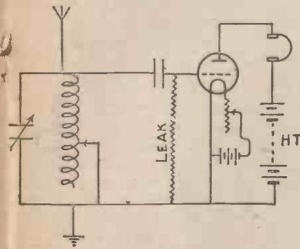
Fig. 9.—Alternative Connections for Grid Leak.
