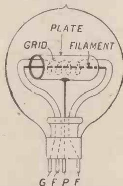
Fig. 9.—Three-electrode Valve shown Diagrammatically.
