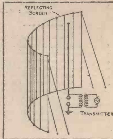
Fig. 13.—Arrangement of Directional Transmitter
