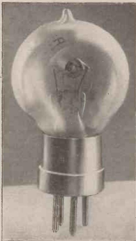
Photograph of Three-electrode Valve.
