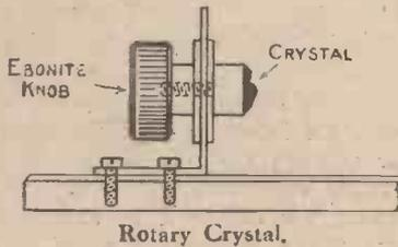
knob the crystal can be moved so that any point on its surface can be touched by the metal contact. This is an improvement on the common ball-and-socket movement, as once the sensitive point is found the crystal is held in position by tightening the knob. J. T. D. W.
