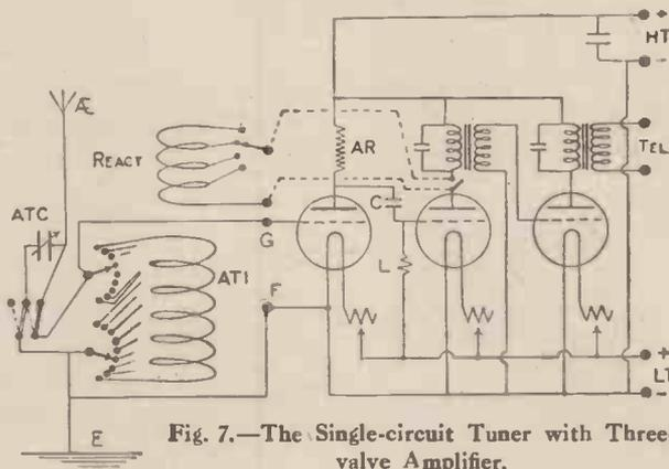
Fig. 7.—The Single-circuit Tuner with Three-valve Amplifier.
