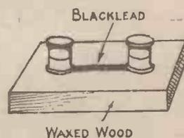
Fig. 5.—Pencil-line Grid Leak.
