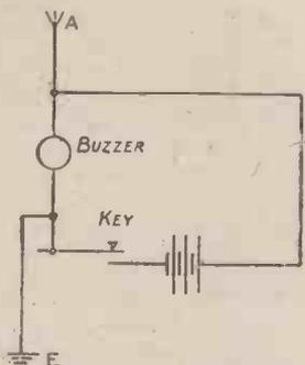
Fig. 2.—Circuit Diagram of Simple Transmitter.
