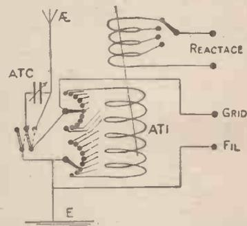
Fig. 6.—The Single-circuit Receiver with "Series-parallel" Condenser and Tapped Reactance Coil.
