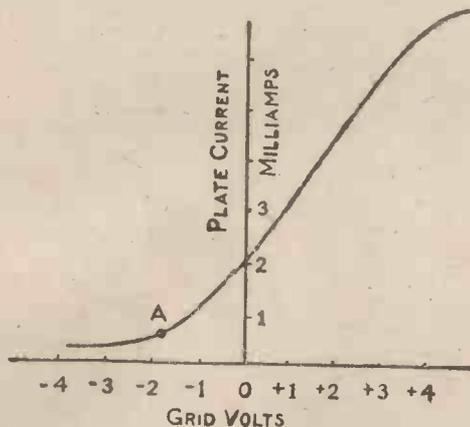
Fig. 1.—Graph showing Characteristic Curve of Valve.
