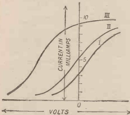
Fig. 11 (right).—Typical Characteristic Curve of a 3-electrode Tube.
