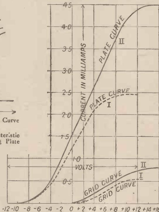
plate circuit, when the grid voltage is progressively increased.
