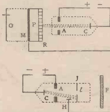
Fig. 4.—Diagrammatic Suggestion of Cathode-ray Transmitting and Receiving Apparatus.
