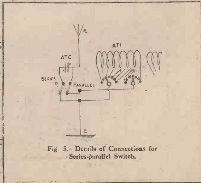
Fig 5.—Details of Connections for Series-parallel Switch.
