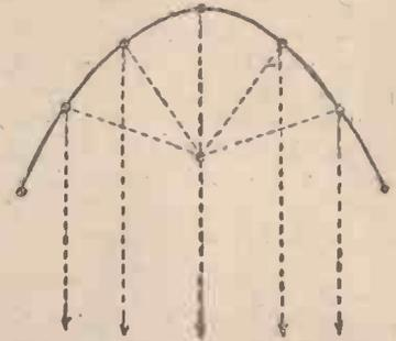
Fig. 2.—Diagram of Beam Projected from a Parabolic Reflector.
