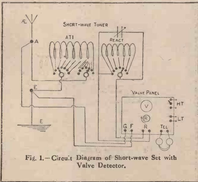
Fig. 1.—Circuit Diagram of Short-wave Set with Valve Detector.
