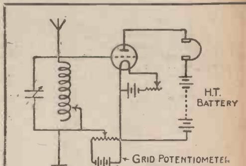
Fig. 2.—Diagram showing Adjustment of Grid Voltage.
