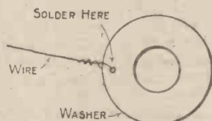
Fig. 5.—Terminal Washer with
