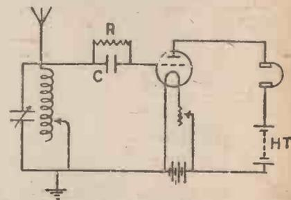
Fig. 3.—Circuit with Condenser and Leak.
