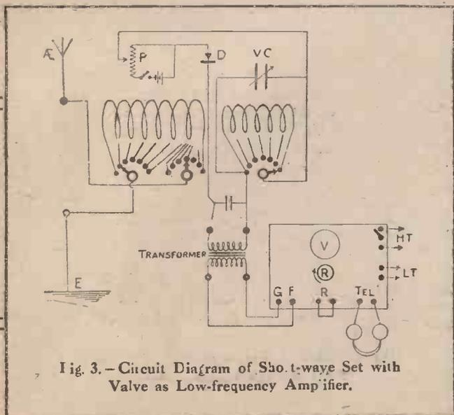
Fig. 3.—Circuit Diagram of Short-wave Set with Valve as Low-frequency Amplifier.
