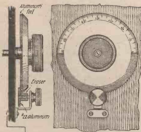
Condenser Shield and Vernier.
