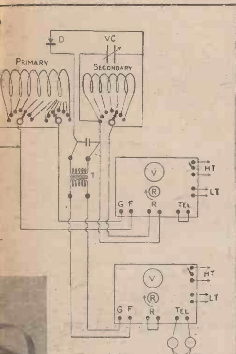
Fig. 4.—Circuit Diagram of Short-wave Set in Conjunction with Two Single-valve Panels.
