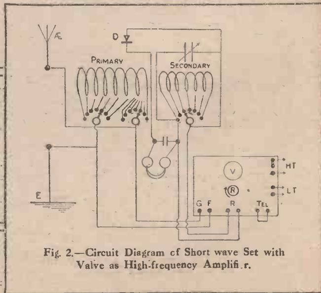
Fig. 2.—Circuit Diagram of Short wave Set with Valve as High-frequency Amplifier.
