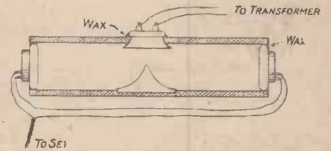
Fig. 1.—Section of Microphone Amplifier.
