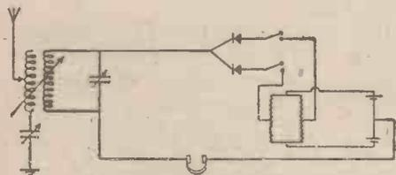
Circuit Diagram for Balanced-crystal Method of Obviating Jamming.
