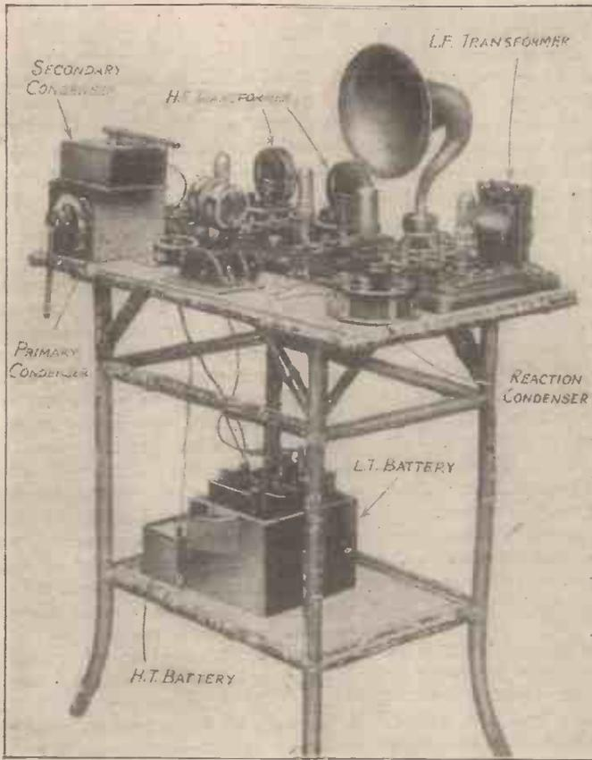
Fig. 2.—Photograph of the Units Arranged as a Four-valve Receiver.
