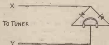
Fig. 2.—Circuit with Two Crystals.
