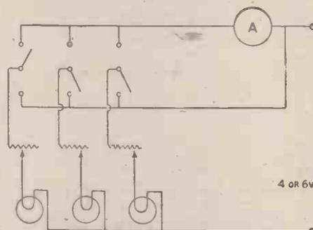
Circuit Diagram showing Arrangement of Switches.
