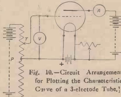
Fig. 10.—Circuit Arrangement for Plotting the Characteristic Curve of a 3-electrode Tube.]
