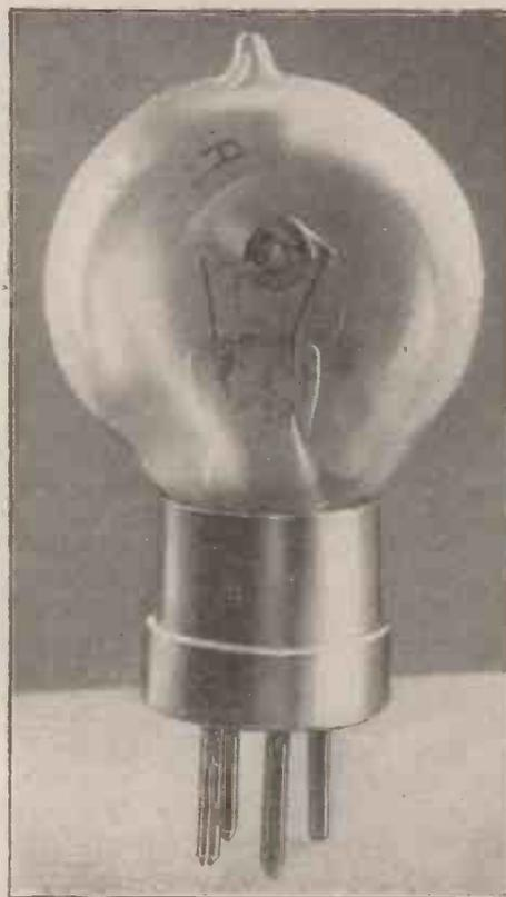
Photograph of Three-electrode Valve.
