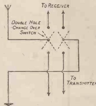
Fig. 3.—Connections of Change-over Switch.
