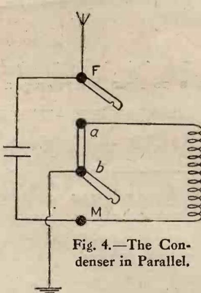
Fig. 4.—The Condenser in Parallel.
