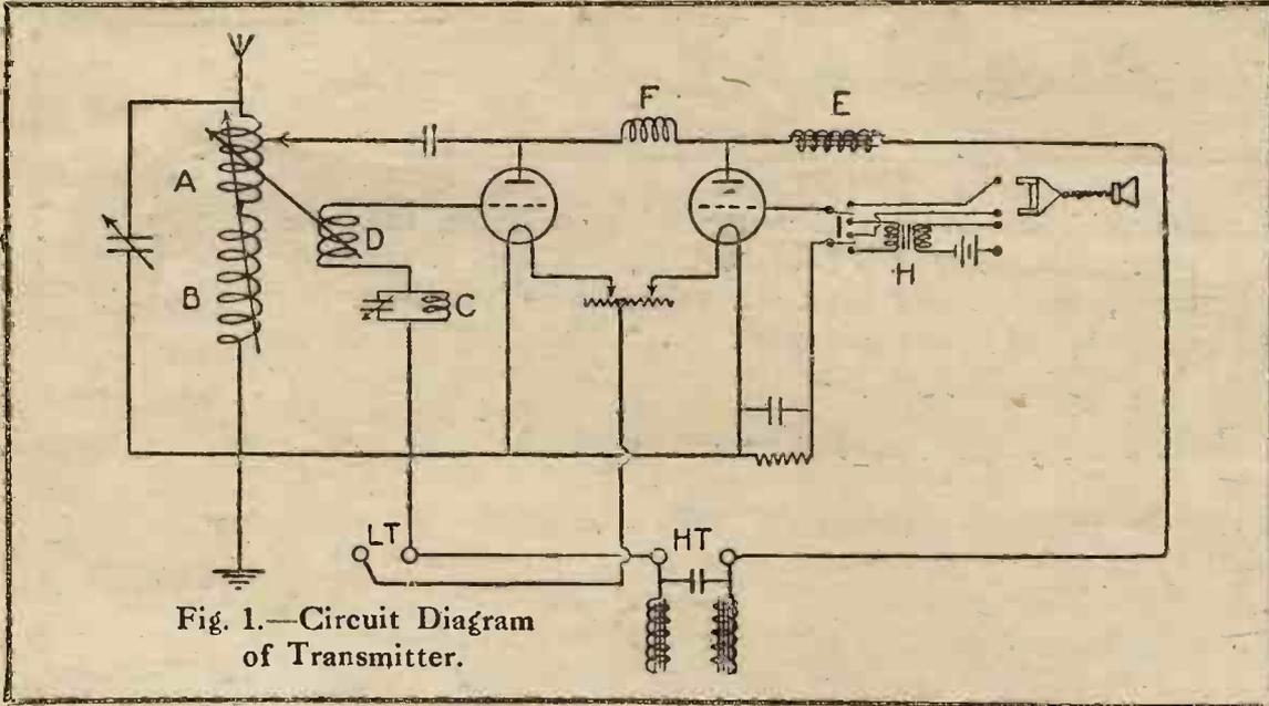
Fig. 1.—Circuit Diagram of Transmitter.
