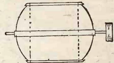
Fig. 3.—Ball-type Rotor (Constant Capacity).
