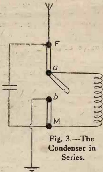
Fig. 3.—The Condenser in Series.
