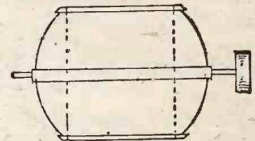
Fig. 3.—Ball-type Rotor (Constant Capacity).
