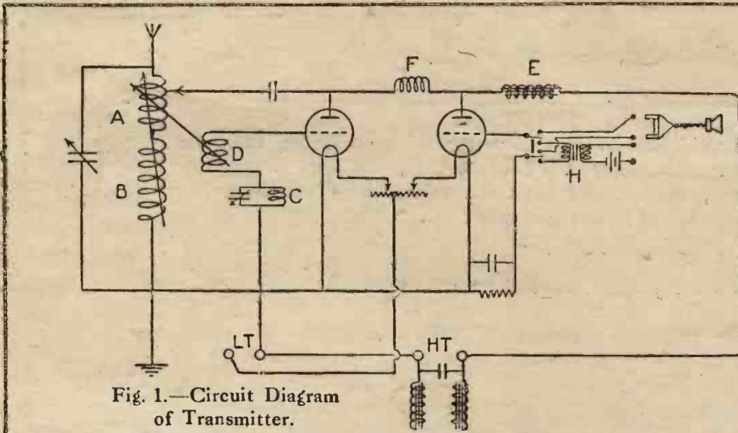
Fig. 1.—Circuit Diagram of Transmitter.
