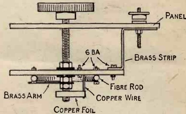
Fig. 3.—Enlarged Detail of Filament Rheostat.
