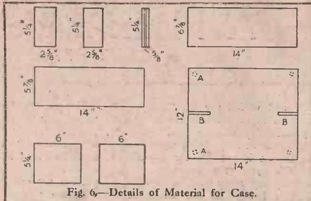
Fig. 6.—Details of Material for Case.
