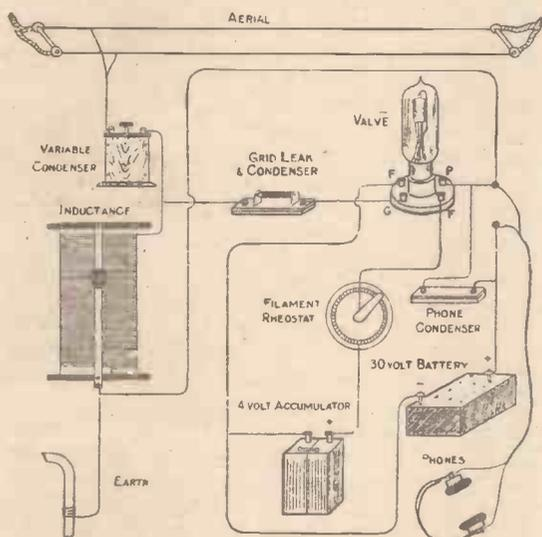
Disposition of Apparatus Corresponding to Diagram Above.
