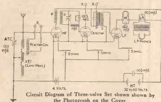
Circuit Diagram of Three-valve Set shown shown by the Photograph on the Cover.
