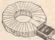
**Burndept Patent Coils** (Patent 168249) are the most efficient for the reception of wireless speech and telephony. In our multi-layer coils, ample air space is provided between each layer, thus ensuring a minimum self-capacity. Coils S. 1 to S. 4 are single layer coils, wound on ebonite, wavelength range 150 to 800 metres.
