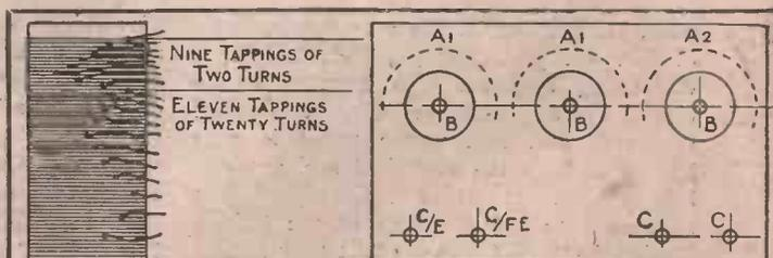
Fig. 2.—Lay-out of Ebonite Panel.
