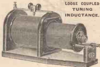
Wavelength range with 100 foot aerial 1,500 metres. Really first-class instrument. Coil ends and base of matt finished ebonite. Secondary tapped in 7 sections with well-made rotary switch. Price 50/-
