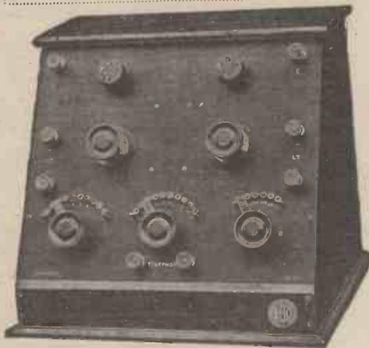
**A TWO-VALVE SET WITH REACTION APPROVED BY POSTMASTER-GENERAL FOR BROADCASTING No. 0236.**
