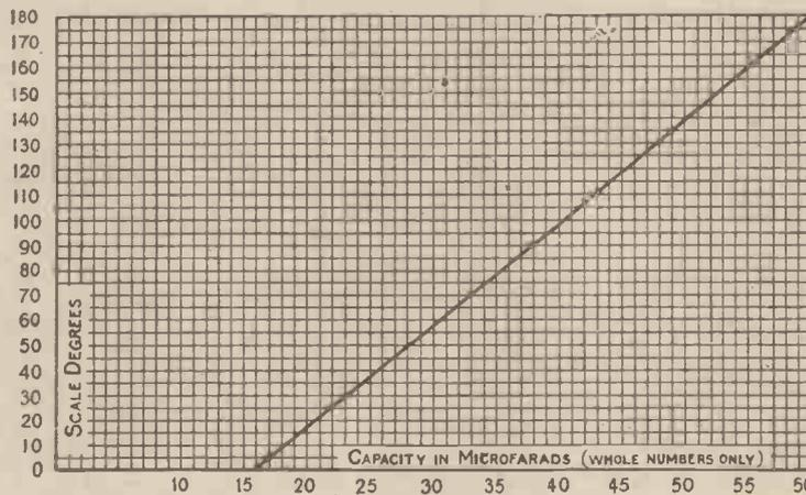
Fig. 1.—Degrees-capacity Chart for .0006 mfd. Condenser.
