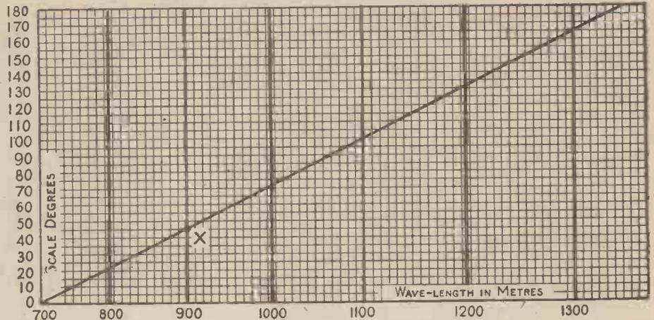
Fig. 2.—Calibration Chart for Inductance Coil.
