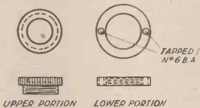
Fig. 2.—Parts of Crystal Cup.
