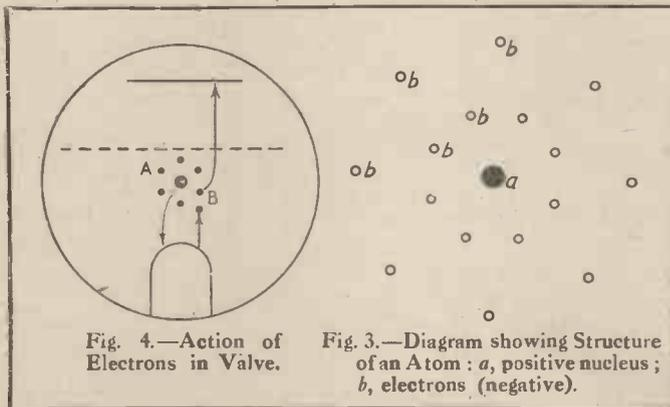
Fig. 4.—Action of Electrons in Valve.
