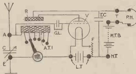
Fig. 4.—Circuit Diagram of Portable Receiver.
