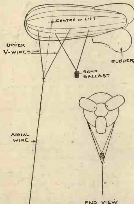
Fig. 2.—Side and End Elevations of Balloon showing Method of Attachment to Line.
