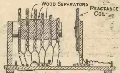
Fig. 2.—Method of Mounting Coils.
