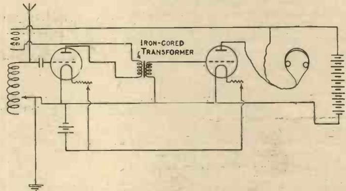
Fig. 4.—Note-magnification Circuit.
