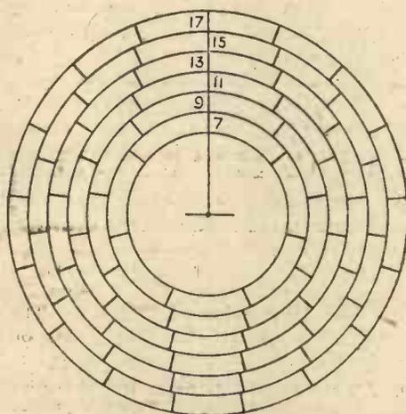
Coil-pin Spacing Diagram.
