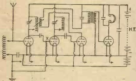
Four-valve Tuned-anode Circuit.
