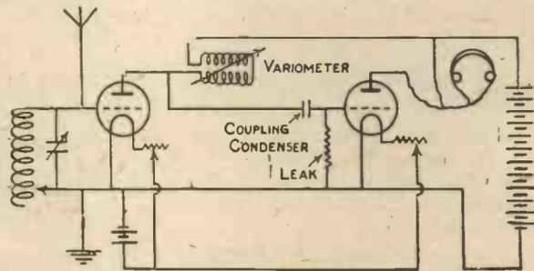
Fig. 3.—Tuned-anode Coupling.
