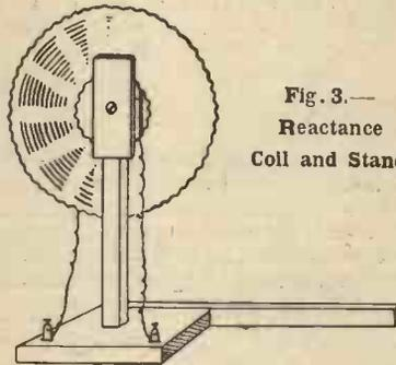
Fig. 3.—Reactance Coil and Stand.
