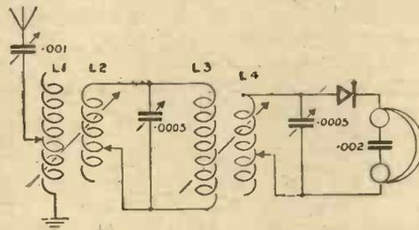
Fig. 14.—A three circuit, or multi-tuner, receiver. Consists of three separate circuits, each of which is tuned to the incoming wavelength. Two loose couplers can be conveniently used in this circuit in conjunction with three variable condensers whose values are given in the diagram.
