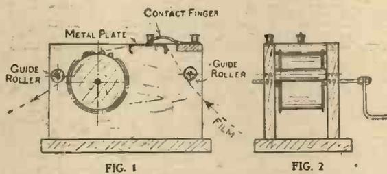
Figs. 1 and 2.—Side and End Elevations of Transmitter.
