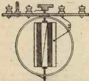
Fig. 1.—Section of Complete Variometer.
