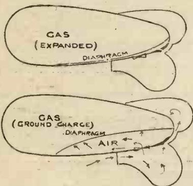
Fig. 1.—Diagrams Explaining Action of Balloonet.
