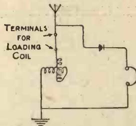
Fig. 3.—Circuit Diagram of Variometer Receiver.
