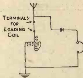
Fig. 3.—Circuit Diagram of Variometer Receiver.
