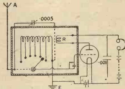
Fig. 4.—Circuit Diagram of Complete Receiver with One Valve Employing Reaction.
