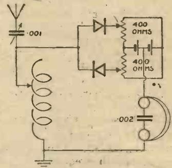
Fig. 13.—A balanced-crystal circuit, useful for experiments in the elimination of atmospheric. It will be seen that the crystals are connected in opposite directions and are connected to the sliders of a double potentiometer. The telephones are placed between the earth terminal and the centre of the 3-volt dry battery across the potentiometer.
