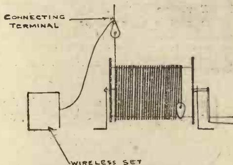
Fig. 3.—Winding Drum and Receiver Connection
