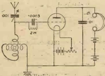
Fig. 16.—Similar to the last except that tuning is carried out by means of a variometer. Here again the series condenser may be omitted, fine tuning usually being quite easy to obtain with the variometer alone. The series condenser, if used, will allow of tuning to a much lower wavelength than would be possible without it.
