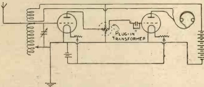
Fig. 2.—Method of Connecting Two Valves with Plug-in Transformer.
