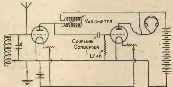
Fig. 3.—Tuned-anode Coupling.
