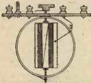
Fig. 1.—Section of Complete Variometer.
