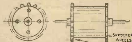
Fig. 3.—Details of Drum.
