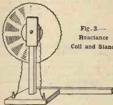
Fig. 3.—Reactance Coil and Stand.
