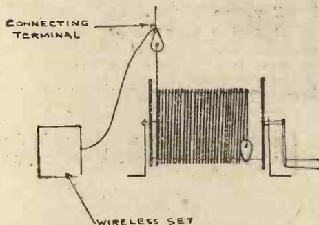
Fig. 3.—Winding Drum and Receiver Connection
