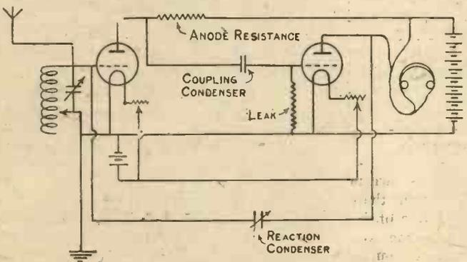
Fig. 5.—Resistance-capacity Coupling.
