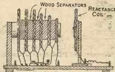
Fig. 2.—Method of Mounting Coils.
