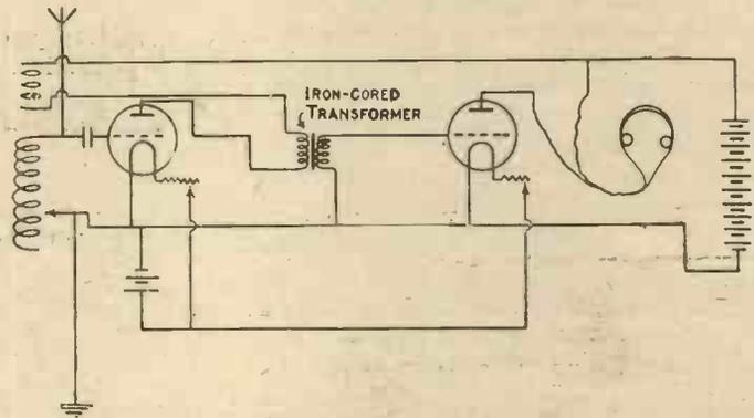
Fig. 4.—Note-magnification Circuit.
