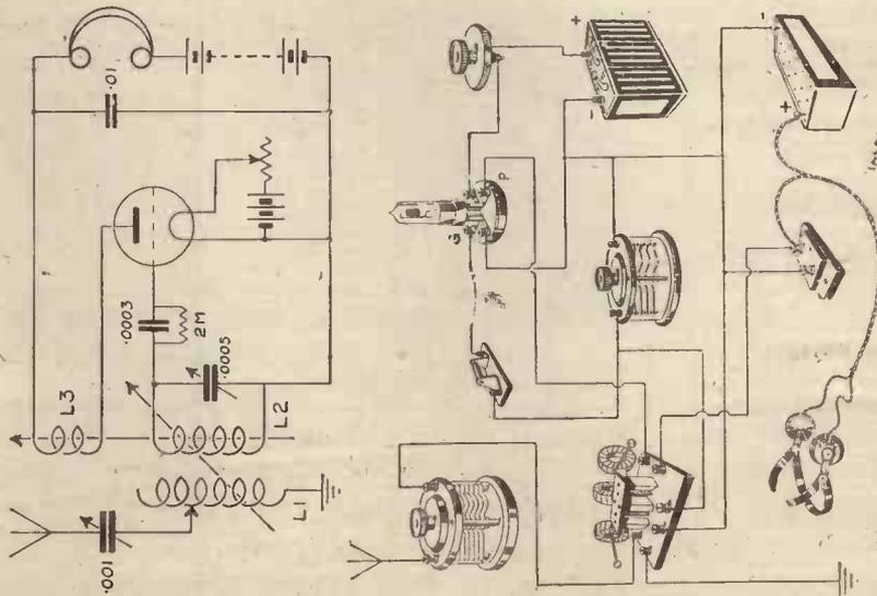
Fig. 22.—Similar to Fig. 21, but a three-coil tuning system is shown. This circuit may be used on broadcast wavelengths provided L1 and L2 are spaced well apart to prevent the reaction coil L3 energising the aerial coil.
