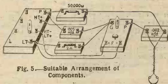
Fig. 5.—Suitable Arrangement of Components.
