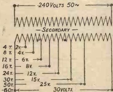
Fig. 2.—Details of Transformer.
