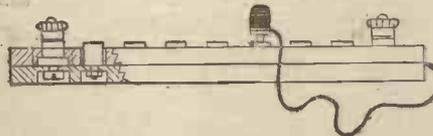
Fig. 5.—The Complete Leak shown in Part Section.
