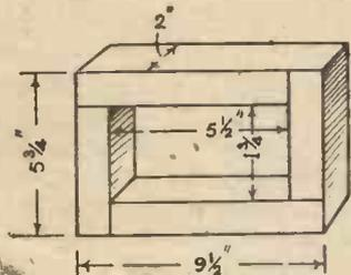
Fig. 1.—Transformer Core.
