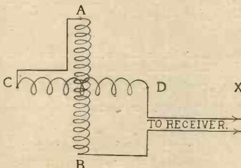
Fig. 1.—Arrangement of Loop Aerials for Maximum Method.
