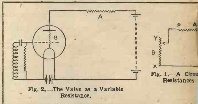
Fig. 2.—The Valve as a Variable Resistance.
