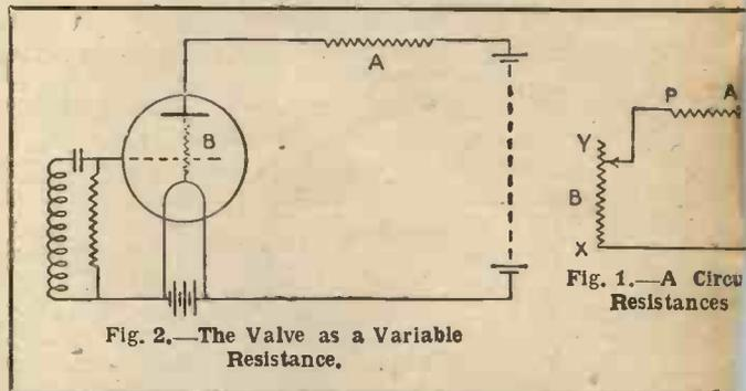
Fig. 2.—The Valve as a Variable Resistance.
