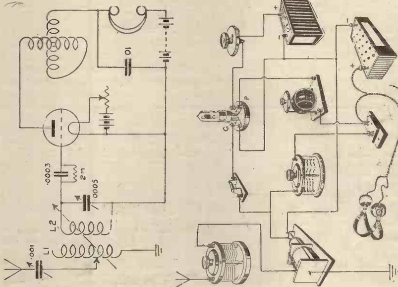
Fig. 23.—A very efficient regenerative circuit for short-waves. The variometer in the plate circuit, if tuned to the frequency of the incoming oscillations, will set the whole system oscillating. If this circuit is used for broadcasting, the variometer should be slightly mistuned.
