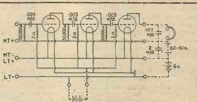
Fig. 4.—Circuit Diagram of Note-magnifier.
