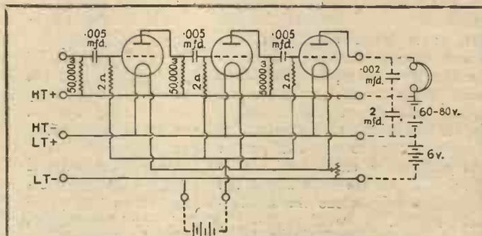
Fig. 4.—Circuit Diagram of Note-magnifier.
