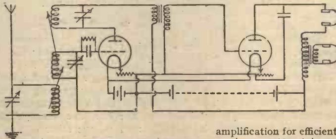
Two-valve Circuit (1 Det. and 1 L.F.) for use with High and Low Resistance Phones.
