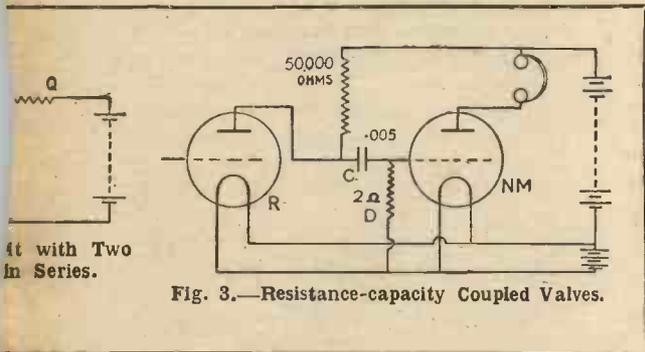
Fig. 3.—Resistance-capacity Coupled Valves.
