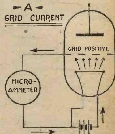
Fig. 4.—Measuring Reverse Grid Current
