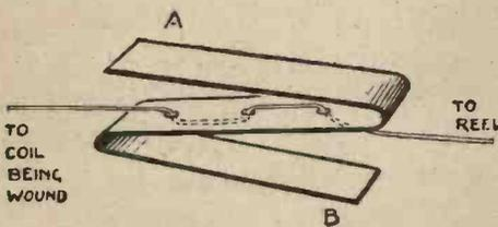
Tool to Simplify Coil Winding.
