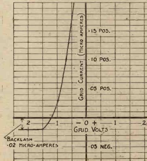
Fig. 5.—Grid-current and Grid-volts Curve (grid current at zero volts = 1 microampere).
