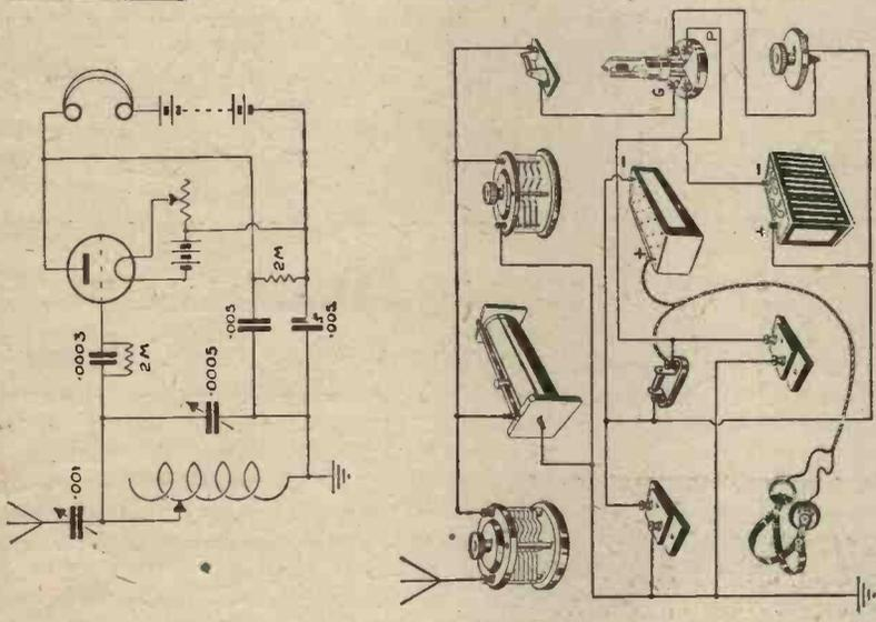
Fig. 32.—Another circuit of American origin. The two blocking condensers in the lower part of the diagram should have a capacity of about .005 microfarad, the leak across them being of a resistance of  $1\frac{1}{2}$  to 2 megohms.
