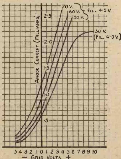
Fig. 3.—Grid-volts and Anode-current Curve.
