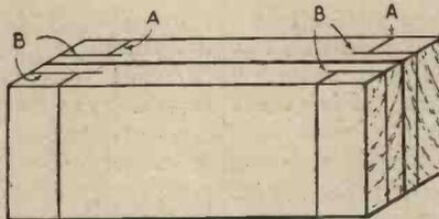
Fig. 3.—Setting-out Dovetailed Joint.
