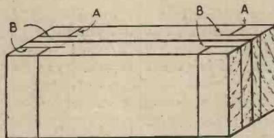
Fig. 3.—Setting-out Dovetailed Joint.
