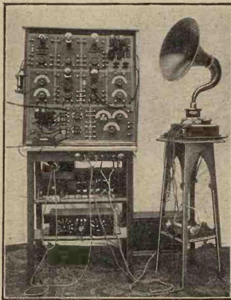
A Five-valve Experimental Receiver constructed from a Peto-Scott Unit Set.
