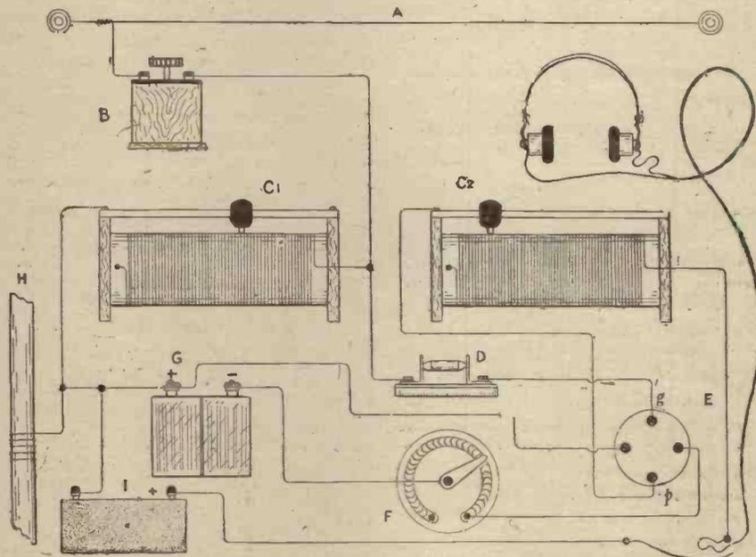
Method of Connecting-up Apparatus for Single-valve Regenerative Receiver.
