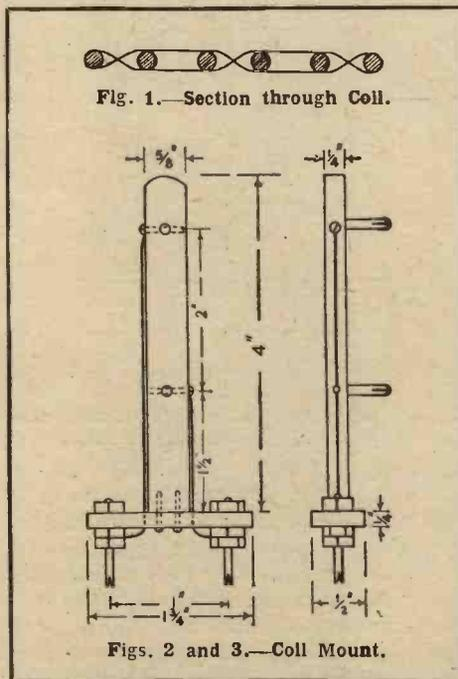
Fig. 1.—Section through Coil.
