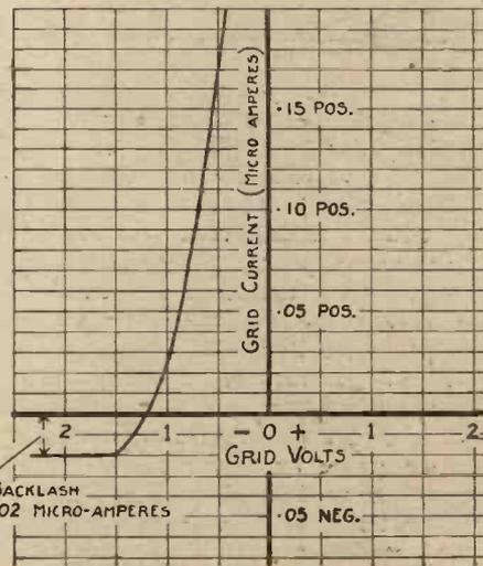
Fig. 5.—Grid-current and Grid-volts Curve (grid current at zero volts = 1 microampere).
