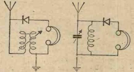
Figs. 2 and 3.—Suitable Crystal Circuits.
