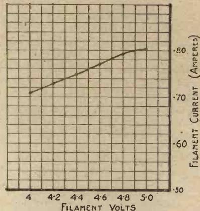
Fig. 2.—Filament-volts and Filament-current Curve.
