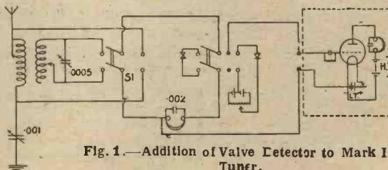
Fig. 1.—Addition of Valve Detector to Mark III Tuner.
