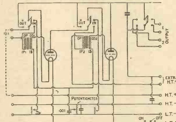
Fig. 1.—Circuit Diagram of Note-magnifier Unit.
