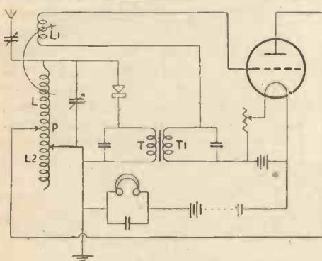
Fig. 8 (left).—Scott-Taggart Dual-amplification Circuit.
