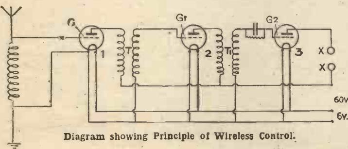
Diagram showing Principle of Wireless Control.
