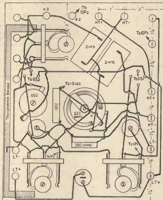
Fig. 2.—Wiring Diagram of Note-magnifier Unit.
