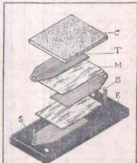
Fig. 2.—Constructional Details of Condenser.
