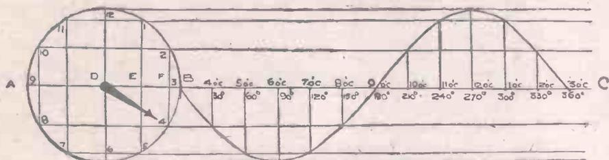
Fig. 4.—Explanation of Sine Wave.
