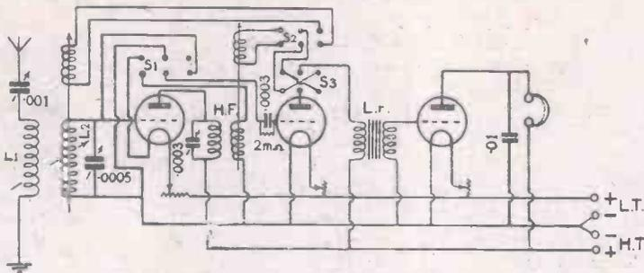
Three-valve circuit with Switching Arrangements.
