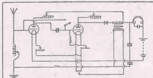
Fig. 1.—Circuit Diagram of Dual-amplification Receiver.
