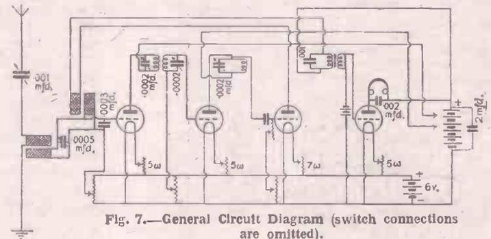
Fig. 7.—General Circuit Diagram (switch connections are omitted).
