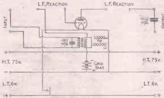
Fig. 6.—Circuit Diagram of Low-frequency Unit.
