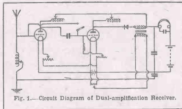
Fig. 1.—Circuit Diagram of Dual-amplification Receiver.
