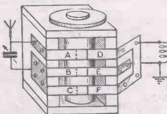
Details of Barrel Switch.
