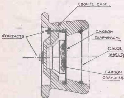
Fig. 1.—Section of Carbon-type Microphone.
