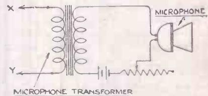
Fig. 2.—Diagram of Microphone Circuit.
