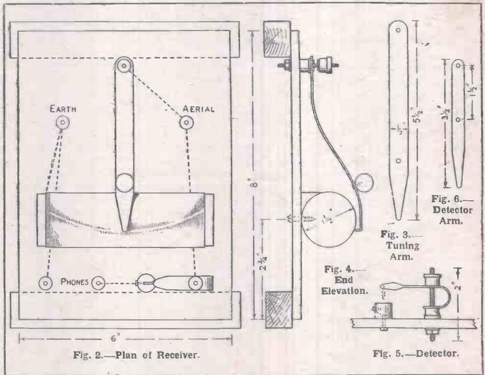
be  $2\frac{3}{4}$  in. from the front edge (Fig. 2). Terminals for aerial, earth and telephones may now also be screwed into position.
