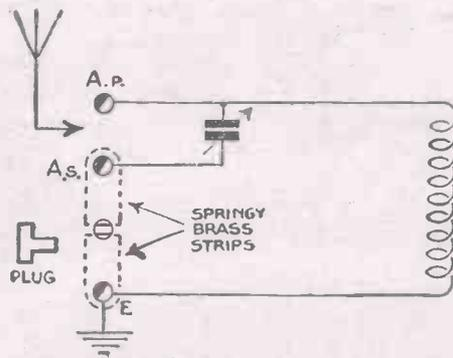
Fig. 6.—Series-parallel Connections.
