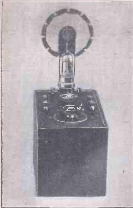
Fig. 4.—The Complete Wavemeter.
