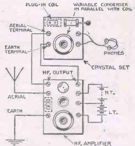
Fig. 6.—Method of Connecting Amplifier to Crystal Set.
