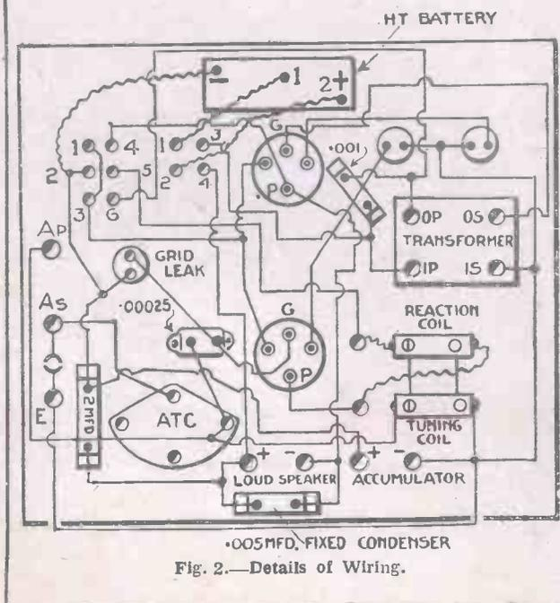
Fig. 2.—Details of Wiring.
