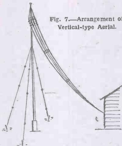
Fig. 7.—Arrangement of Vertical-type Aerial.
