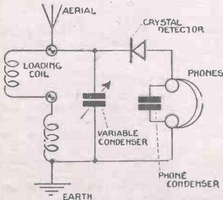
Fig. 3.—Should it be desired to receive on long wavelengths, a loading coil can be inserted as shown above. Note that the variable condenser is connected across both coils.
