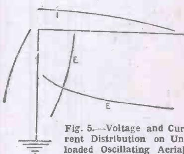
Fig. 5.—Voltage and Current Distribution on Unloaded Oscillating Aerial.
